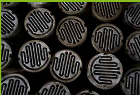
Newly manufactured clay cooking devices are laid out to dry before electric coils are fitted onto them, in a workshop in Bhaktapur, Nepal. Credit: REUTERS/Navesh Chitrakar
