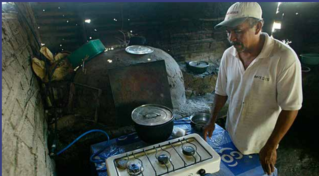
A man watches his stove light, fueled by his household biogas system, which runs on cow manure. Guazapa, El Salvador. Credit: REUTERS/Luis Galdamez
