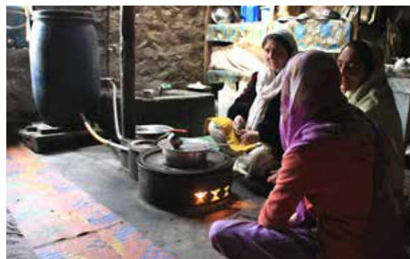
Improved stoves that cook, heat water and warm homes in Northern Pakistan. Credit: Aga Khan Planning and Building Service (AKPBS) project, Ashden Awards.
