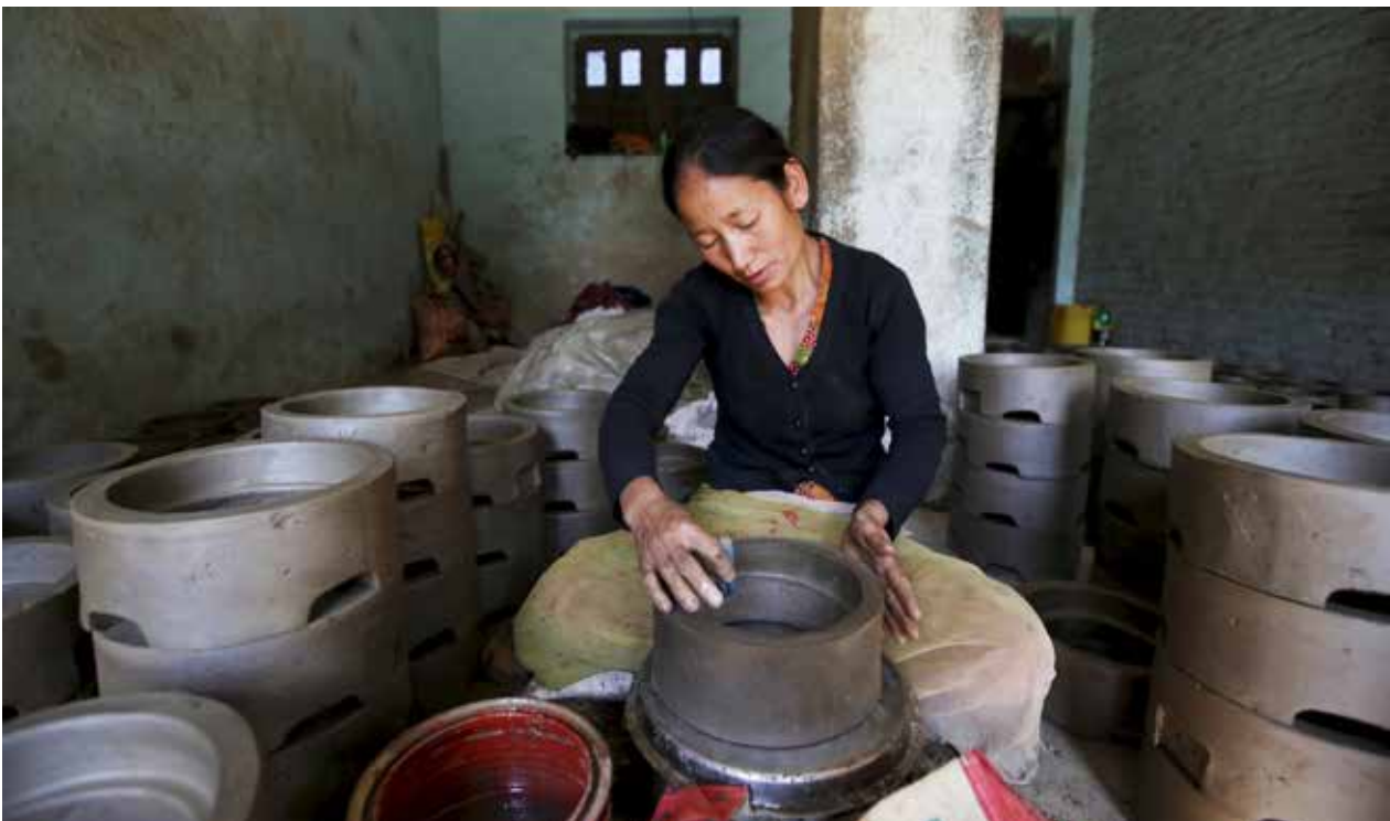
A worker fashions the body of an electric cooking device out of clay in Bhaktapur, Nepal. Demand for electric cookers has risen in the midst of fuel shortages in Nepal.
