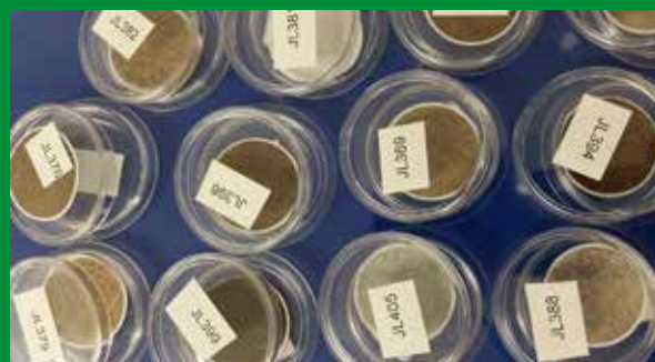
Filter papers collected from homes to monitor household air pollution in Uttarakhand, India. Credit: Jessica Lewis
