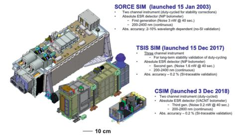
\* The evolution of the solar spectral irradiance monitor (SIM) from SORCE to TSIS to CSIM where the size and mass of the latter were reduced to fit into a 6U CubeSat.
