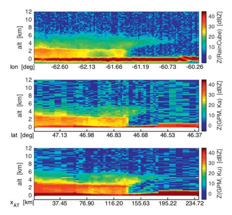
\* Observations along a ~130-km path through a large stratiform precipitation weather system near Prince Edward Island, Canada, on 25 Jan 2019. The radar cross sections of Ka-band RainCube radar and that of the GPM DPR were within 9 min from each other. The DPR operates at two frequencies: 14 (Ku) and 35 (Ka) GHz. These matches were done by maximizing feature matching between the RainCube curtain and the DPR 3D volume scans.
