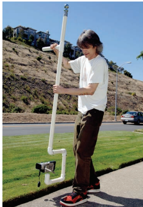
Shaky handheld footage is so 1990s—shoot smooth handheld footage with a home-brew Steadicam.
