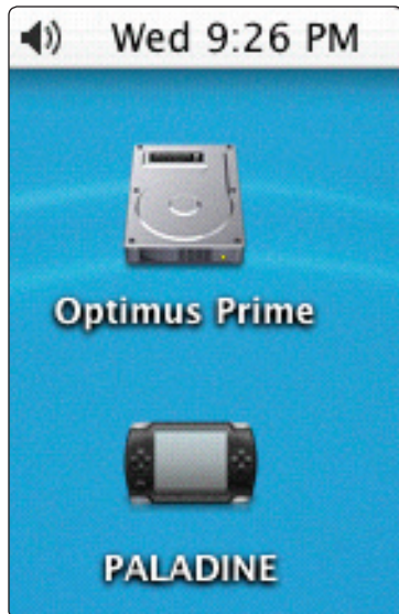
The PSP (we call ours Paladine) mounts on the desktop like a removable volume—but only after you supply a USB cable.
