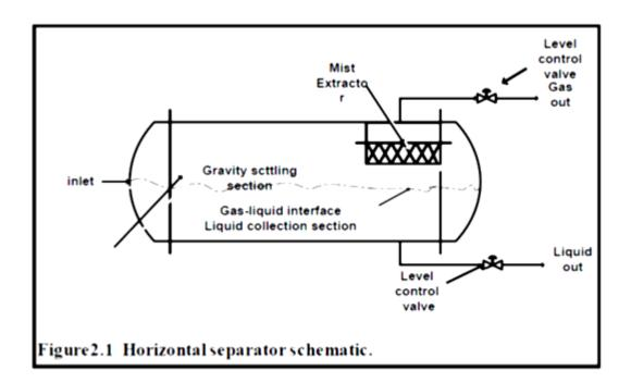
The pressure in the separator is maintained by a pressure controller. The pressure controller senses changes in the pressure in the separator and sends a signal to either open or close the pressure control valve accordingly. By controlling the rate at which gas leaves the vapor space of the vessel the pressure in the vessel is maintained. Normally, horizontal separators are operated half full of liquid to maximize the surface area of the gas liquid interface.
