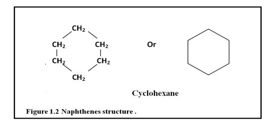
The boiling point and densities of naphthenes are higher than those of alkanes having the same number of carbon atoms. Naphthenes commonly present in crude oil are rings with five or six carbon atoms.
