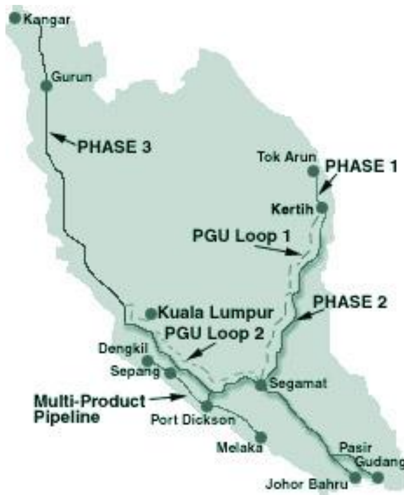
Figure 57 Malaysia Peninsular Gas Utilisation System
