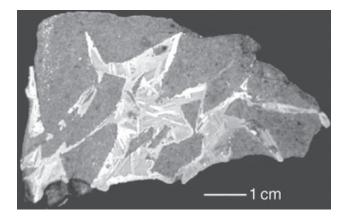
**Fig. 4.** Slice of the Portales Valley meteorite showing dark angular clasts of what appears to be an H6 chondrite separated by light-colored veins of metallic Fe,Ni, which have been etched to reveal a Widmanstätten pattern of oriented kamacite plates. An impact created the angular clasts but it is not known how the molten metal was formed, mixed with chondritic clasts, and then cooled slowly to form the Widmanstätten pattern. (Photo courtesy of Marvin Killgore.)
