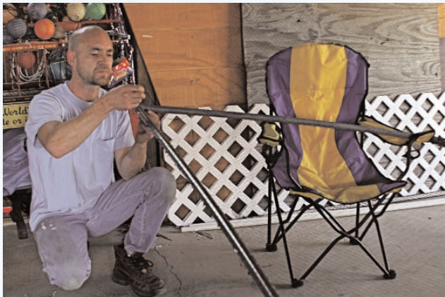
Hook the netting over the screw heads on the frame, stretching the netting taut.
