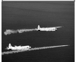
VP-45 P3s Firing ZUNI (5") Rockets
