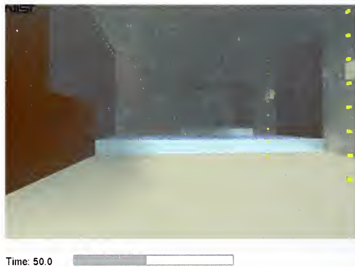
Figure 5-25. Fire suppression continues in both the experiment and the simulation, t = 50 seconds after ignition.
