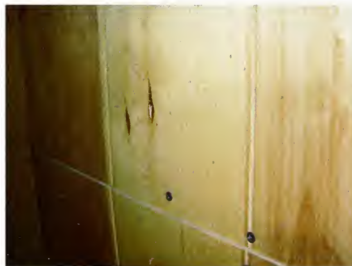
Figure 4-14b. Damage to wood panel following impingement by sparks from gerb. Lip on panel surface can be seen as line below mounting screws.
