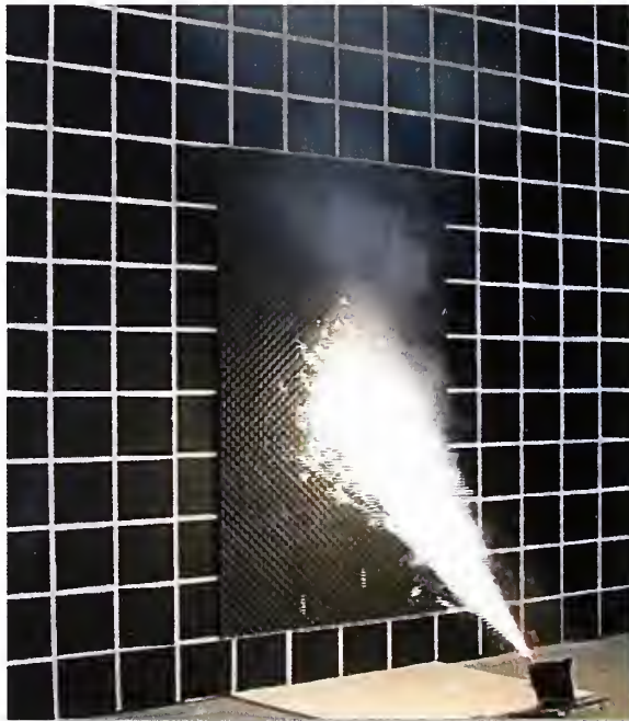
Figure 4-13f. Standard and Infrared Video Images of Gerb Discharge onto a Non-fire Retarded Polyurethane Foam Sheet on Gypsum Board Wall at t = 10 seconds.
