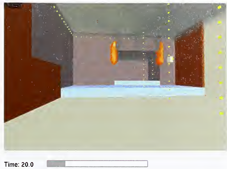
Figure 5-21. Flames impinging on ceiling, t = 20 seconds after ignition.
