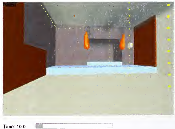
Figure 5-20. Flames spreading toward ceiling, t = 10 seconds after ignition.
