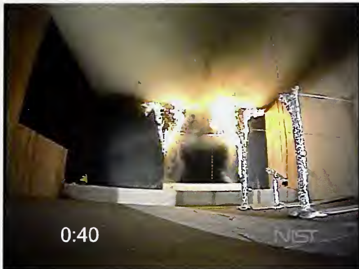
Figure 5-6. Flames continue to spread into alcove, t = 40 seconds after ignition.
