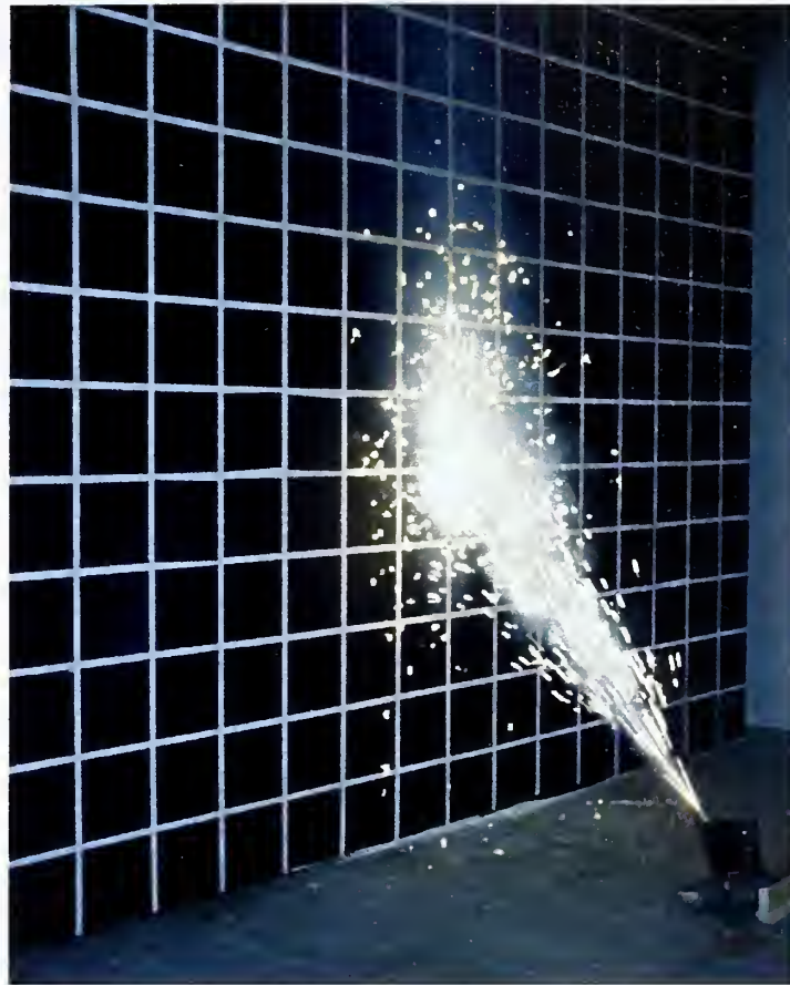
Figure 4-11. Single Gerb at 45 degrees and in a Plane Perpendicular to Wall.
