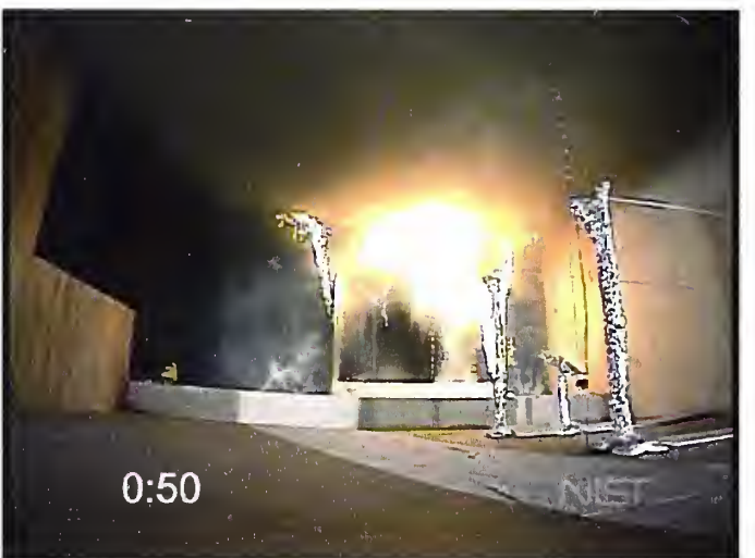
Figure 4-20. Still frames taken from video of full-scale mock-up experiments. Time after ignition is indicated in lower left of each frame. Left column: unsprinklered; right column: sprinklered (first head activates at 24 seconds)
