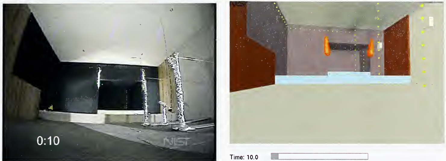
Figure 5-3. Flames spreading toward ceiling, t = 10 seconds after ignition.
