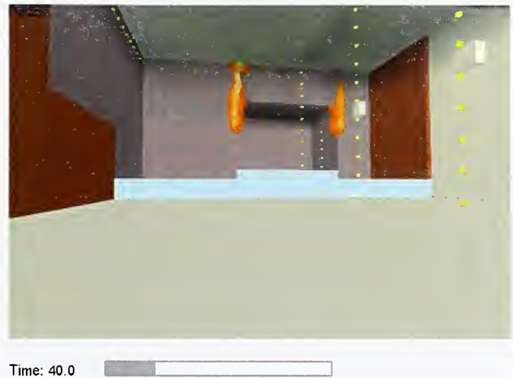
Figure 5-6. Flames continue to spread into alcove, t = 40 seconds after ignition.
