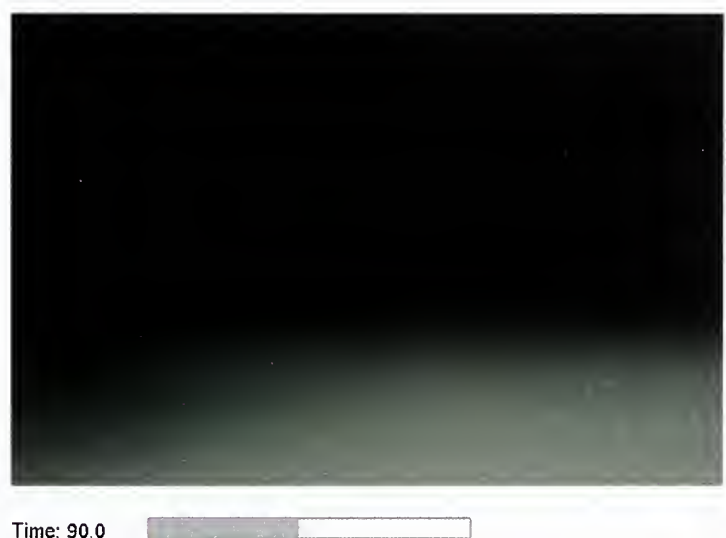
Figure 5-11. Visibility lost, t = 90 seconds after ignition.
