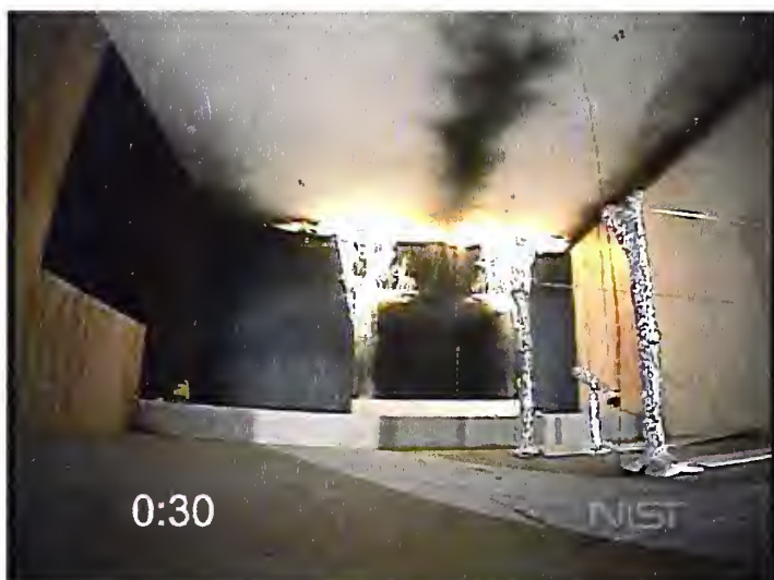
Figure 5-5. Visible smoke spreading across ceiling, t = 30 seconds after ignition.
