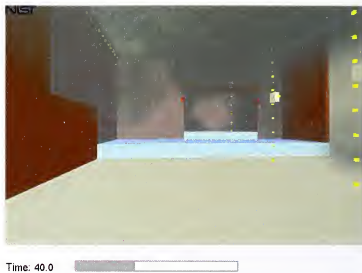
Figure 5-24. Suppression with three sprinklers operating in each case, t = 40 seconds after ignition.
