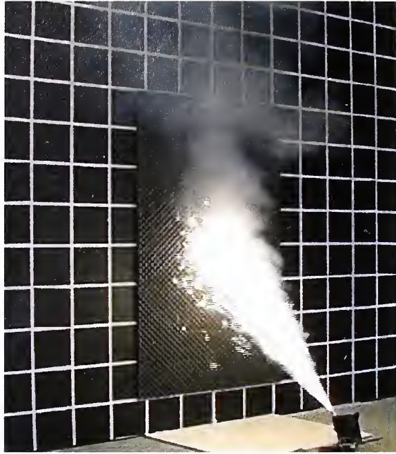
Figure 4-13e. Standard and Infrared Video Images of Gerb Discharge onto a Non-fire Retarded Polyurethane Foam Sheet on Gypsum Board Wall at t = 5 seconds.
