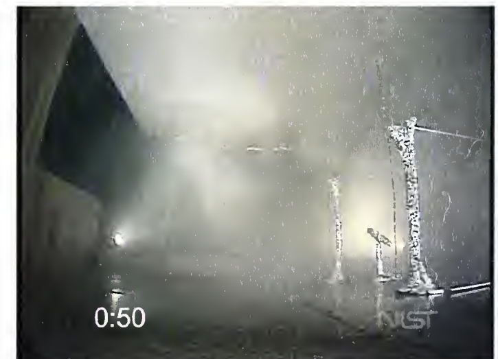
Figure 4-20. Still frames taken from video of full-scale mock-up experiments. Time after ignition is indicated in lower left of each frame. Left column: unsprinklered; right column: sprinklered (first head activates at 24 seconds)
