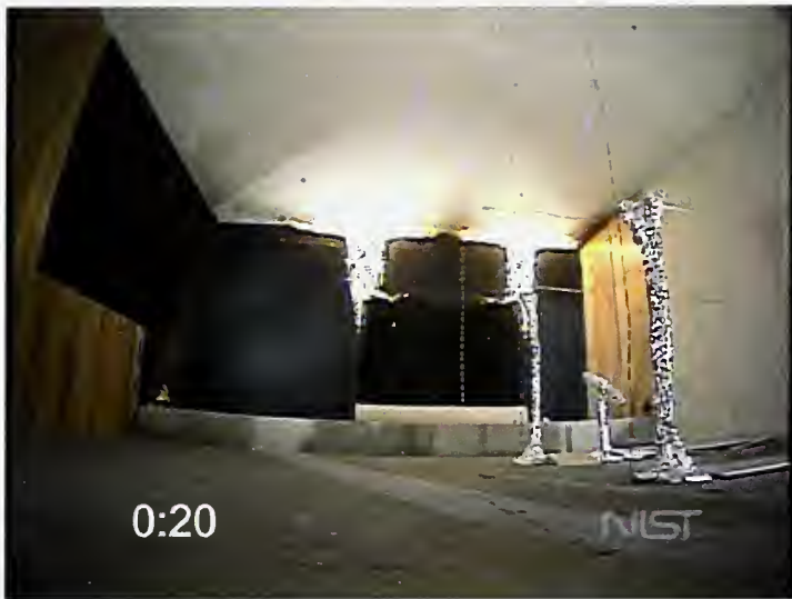
Figure 5-21. Flames impinging on ceiling, t = 20 seconds after ignition.
