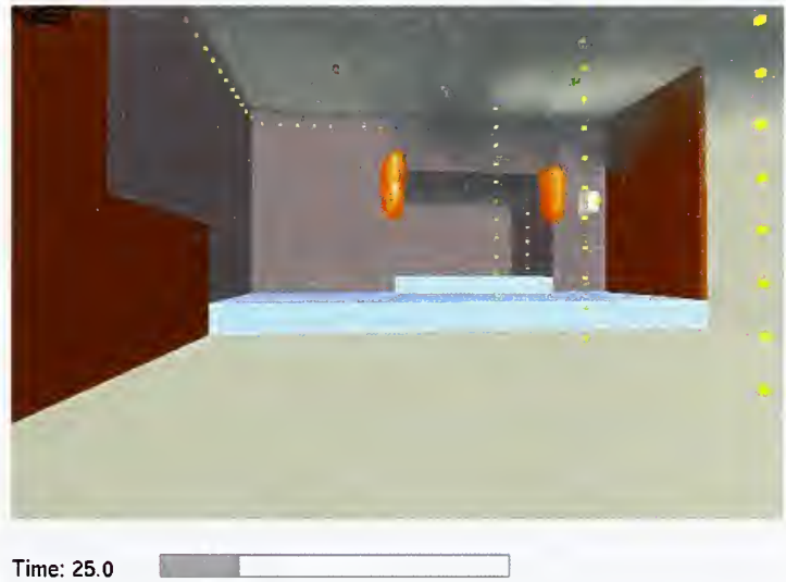
Figure 5-22. Initial sprinkler operating, t = 25 seconds after ignition.
