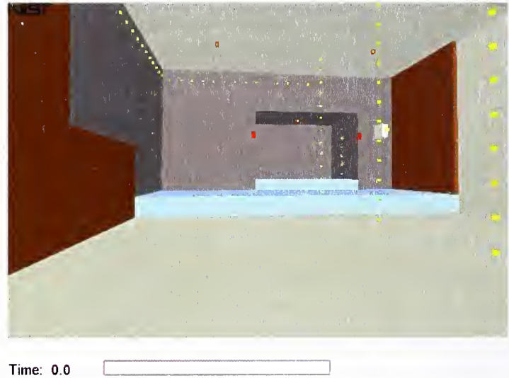
Figure 5-19. Ignition at the corners of the alcove, t = 0 seconds.
