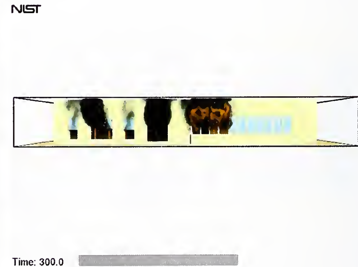
Figure 5-52. Flames breaking through front door and sunroom windows (337 seconds video, 300 seconds simulation)
