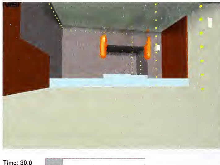
Figure 5-5. Visible smoke spreading across ceiling, t = 30 seconds after ignition.
