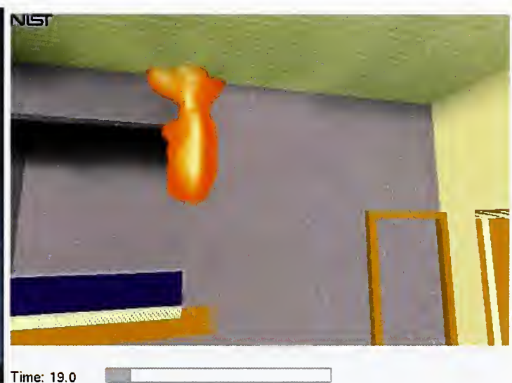
Figure 5-44. Flames impinging on ceiling (19 seconds)
