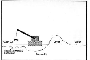
Step 1: Dredge excavates additional material from borrow pit or salt pond bottom adjacent to borrow pit.
