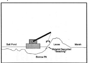
Step 2: Dredge deposits excavated material on levee at water line (referred to as "beaching").
