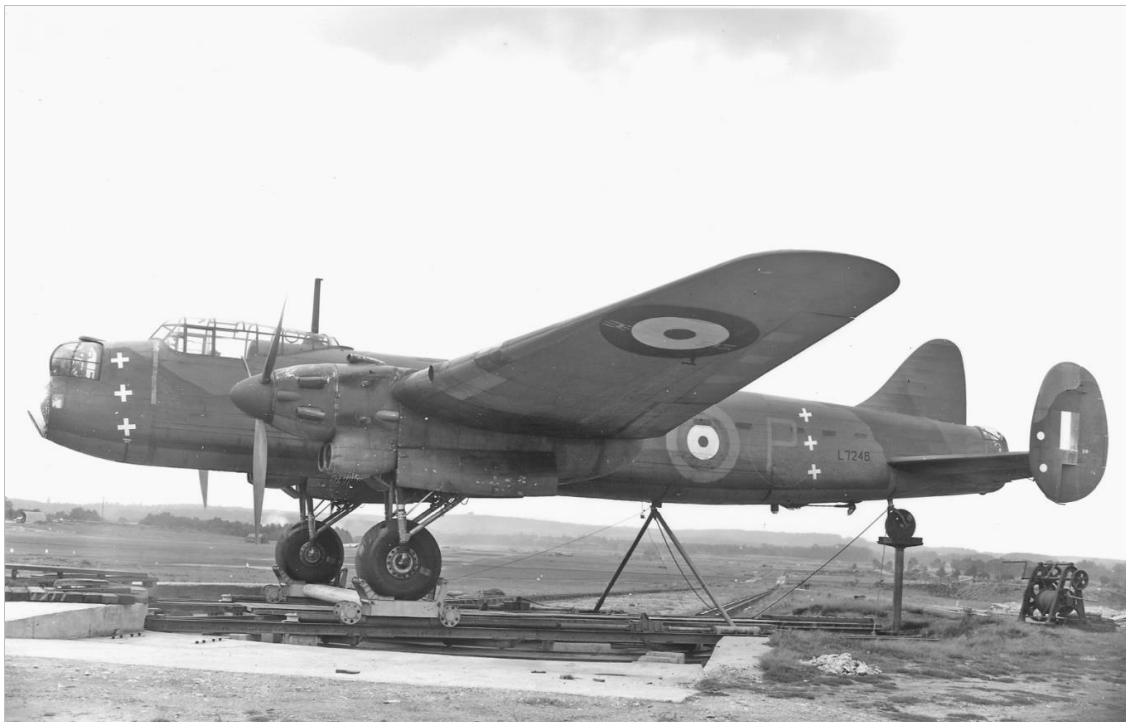
Figure 41. The underpowered Avro Manchester prototype mounted on the catapult prior to being turned into wind for experiments into accelerated take-off.
