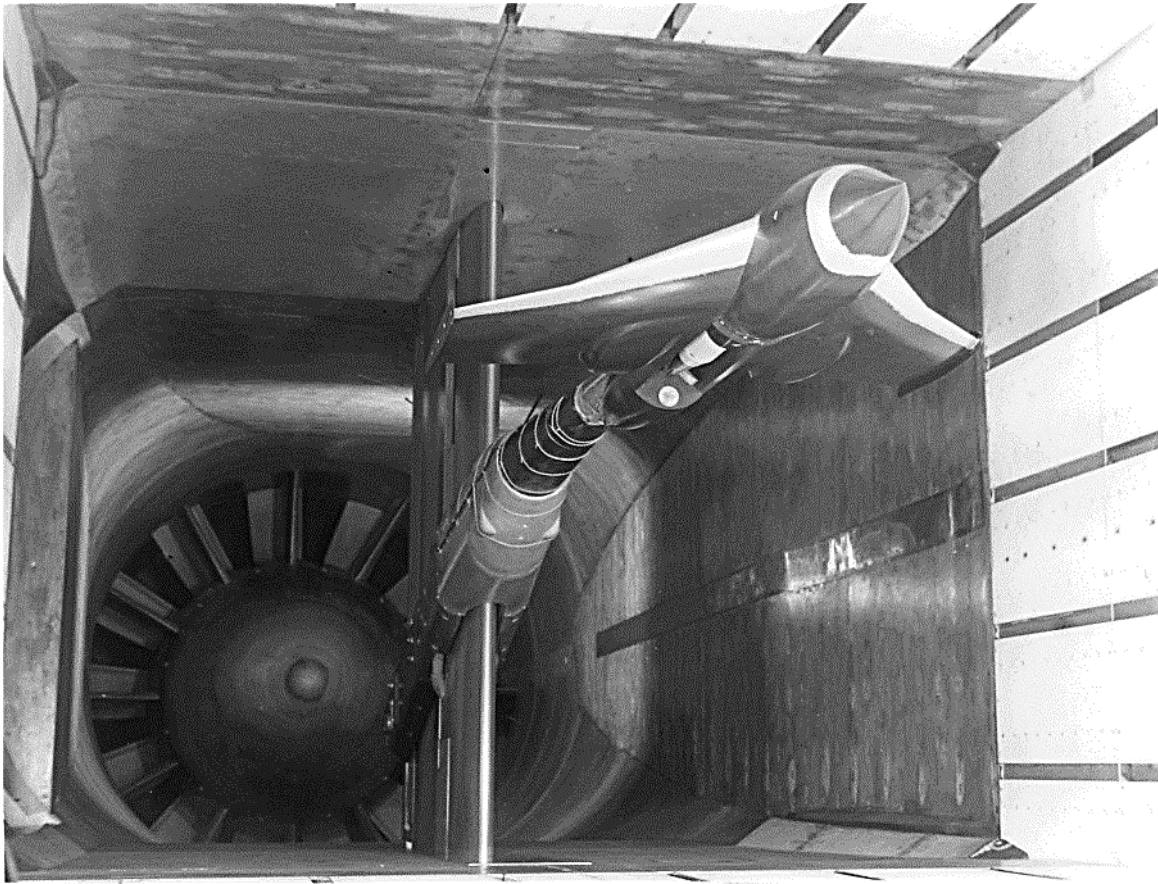
Figure 23. A model of the Handley Page Victor carrying a 'Yellow Sun' atomic weapon runs in the Transonic Tunnel to measure the potential aerodynamic interactions experienced during weapon release.
