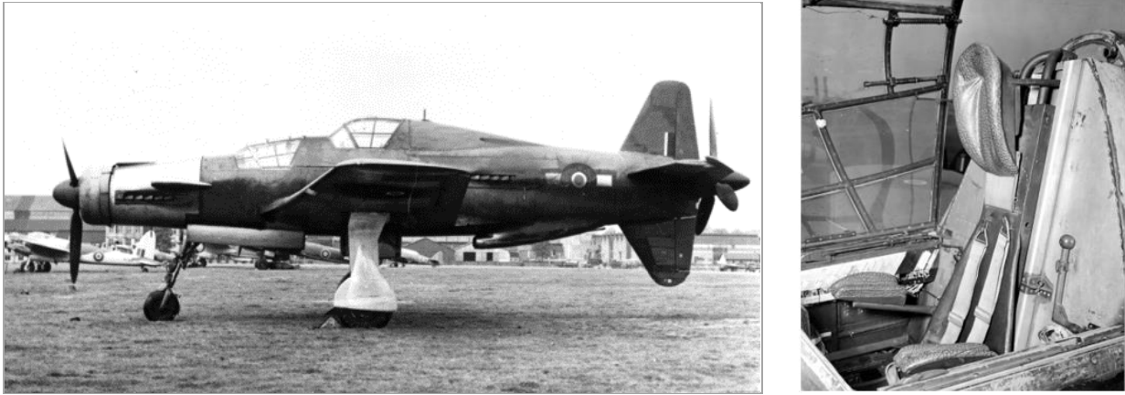
Figure 37. The Enemy Aircraft Dept. flew this Dornier 335 which was fitted with a production ejection seat
