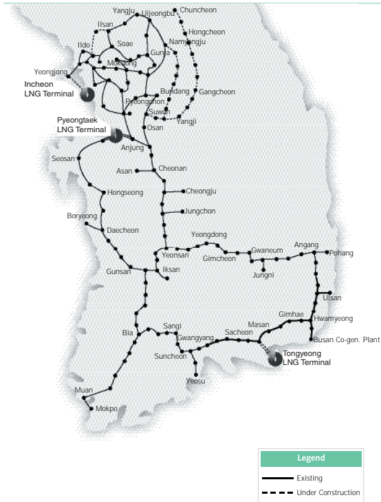
Figure 5.2: South Korea's Natural Gas Grid
