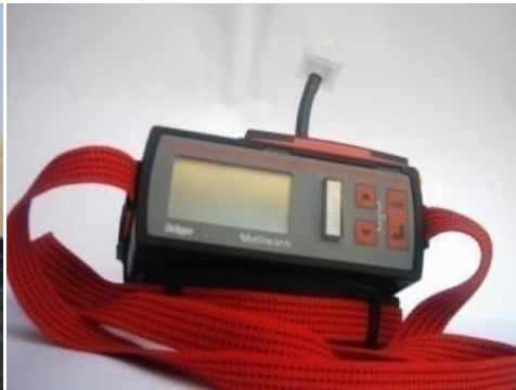
Gas analyzer Drager-Multiwarn/ Germany
