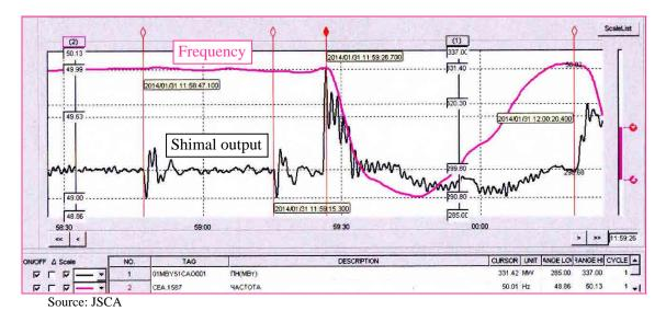
Figure 7.1-16 Frequency and Power Swing in the Case of a Tripped Janub PP
