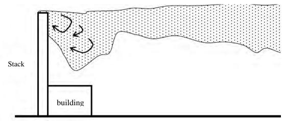
Figure 13.6-5 Diagram of Downwash
