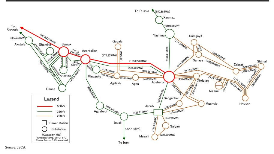
Figure 7.1-5 Network Configuration and Transmitting Capacities
