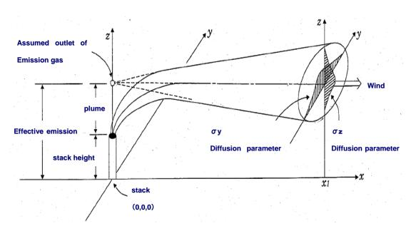
Figure13.6-3 Gaussian Diffusion Model Diagram
