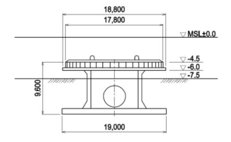
Figure 13.6-10 Water Intake Structures
