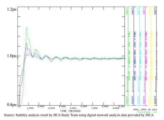
Figure 7.1-14(2) Voltage Fluctuation Curve of Case8
