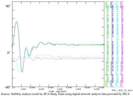
Figure 7.1-15(1) Phase Fluctuation Curve of Generator Voltage of Case11
