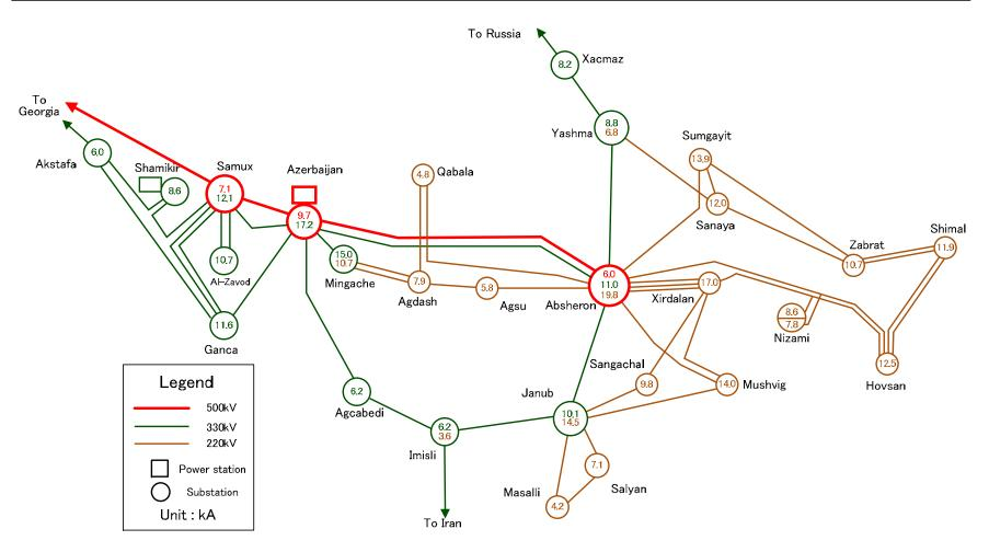
Source: Fault current analysis result by JICA Study Team using digital network analysis data provided from JSCA
