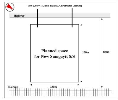
Figure 7.2-10 Planned Construction Site for Sumgayit (STP) S/S
