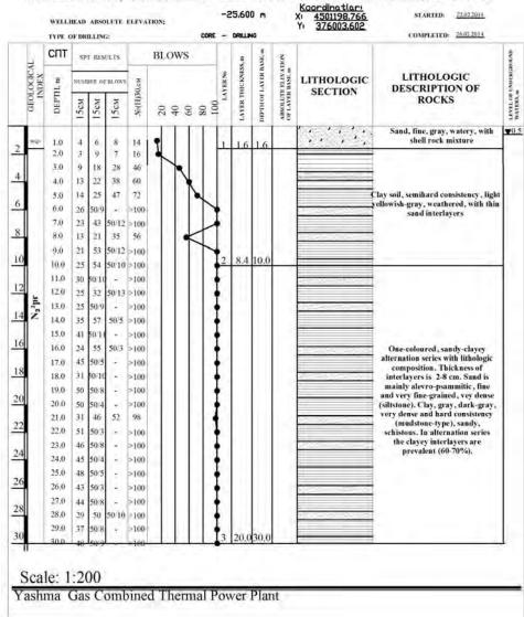
BOREHOLE No6, COLUMN AND THE RESULTS OF DYNAMIC PROBING TEST
