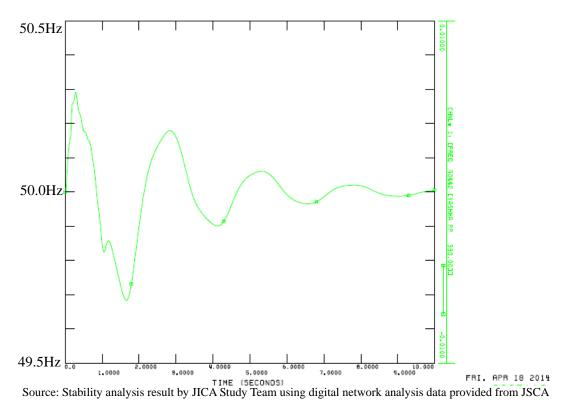
Figure 7.1-15(3) Frequency Fluctuation Curve of Case11
