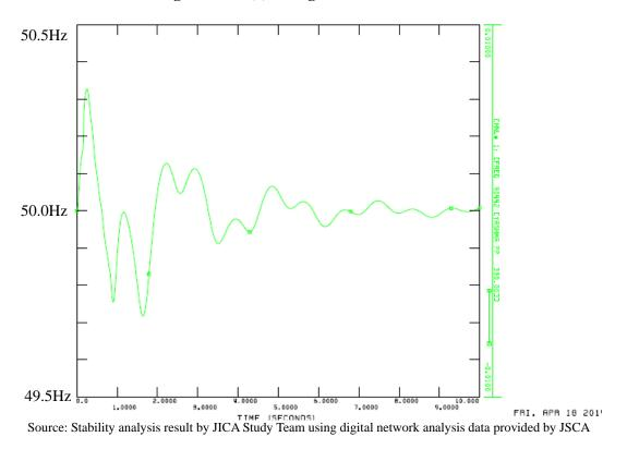
Figure 7.1-14(3) Frequency Fluctuation Curve of Case8
