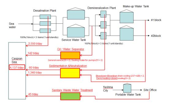
Figure 13.6-14 Waste Water Flow Diagram
