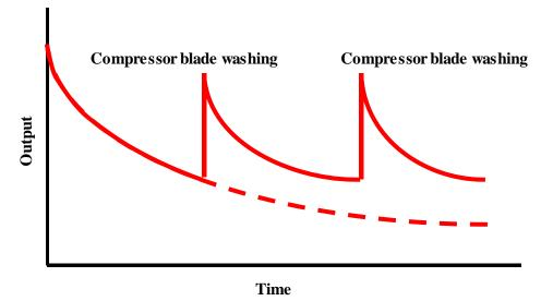
Source: Study Team Figure 11.2-2 Conceptual View of the Compressor Blade Washing Efficiency
