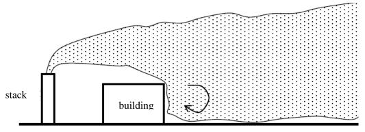
Figure 13.6-4 Diagram of Downdraft
