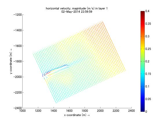
Figure 13.6-16(2) Flow Condition with Thermal Effluent (The future : Current speed 0.3m/s: SE)
