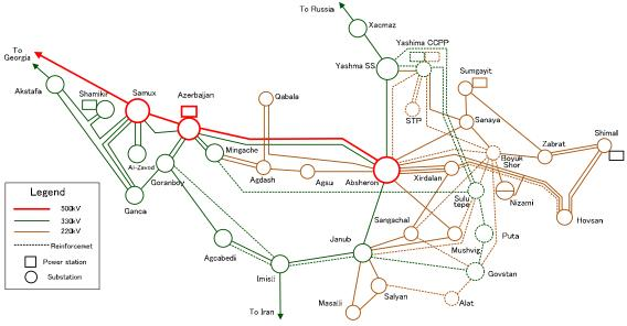
Source: Network analysis data provided by JSCA Figure 7.1-10 Azerenerji JSC's Network Reinforcement
