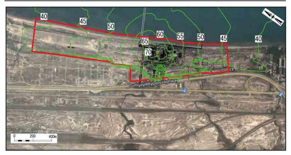
Figure 13.6-15 Results of Simulating Noise Level from Power Plant
