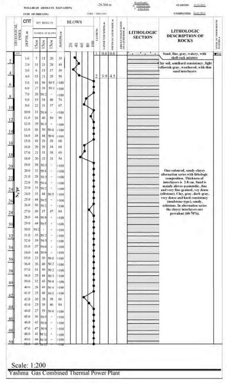
BOREHOLE No1, COLUMN AND THE RESULTS OF DYNAMIC PROBING TEST
