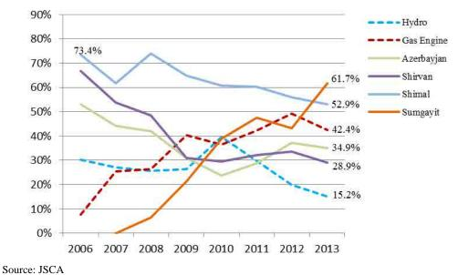
Figure 3.3-2 Load Factor of Each Power Plant
