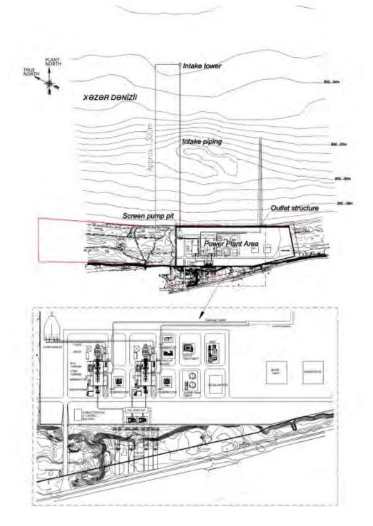
Figure 13.6-9 Intake Tower and Outlet of Cooling Water
