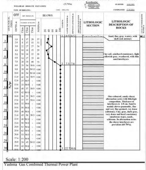
BOREHOLE No5, COLUMN AND THE RESULTS OF DYNAMIC PROBING TEST
