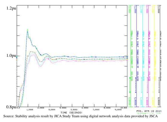
Figure 7.1-15(2) Voltage Fluctuation Curve of Case11
