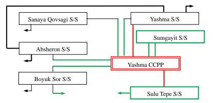
Figure 7.2-1 Grid Connection Plan of Transmission Lines
