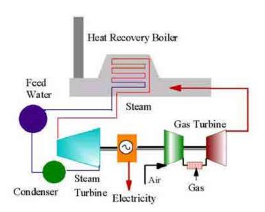
Figure 13.3-2 Mechanism of Combined Cycle Power Generation
