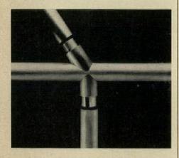
flush-type pipe railings without welds or exposed fasteners. Unlike conventional cast-aluminum fittings, the new connectors allow perfect color matches with pipe, even after alumiliting. Structural soundness and proper alignment are enhanced, since posts and top rails run in continuous lengths, uninterrupted by cross- and tee-fittings. Complete system, with all
