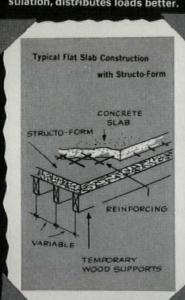
Structo-Form\* provides uniform, lightweight, strong building planks for flat slab or reinforced concrete construction, producing a handsome finished celling.
