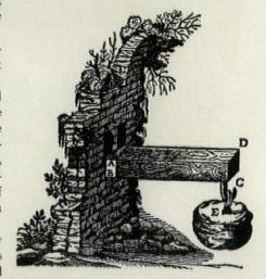
and loading the free end with a large stone. It must be remembered that at this early date his only measuring instruments were his own two eyes. Thus, at the instant of failure, he observed the beam fibers rupturing at A and quickly propagating down to B. This led him to the following conclusion: "It is clear that fracture will occur at the point B, where the edge of the mortise acts as a fulcrum
