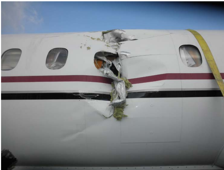
Figure 2 Damage to left side of fuselage
