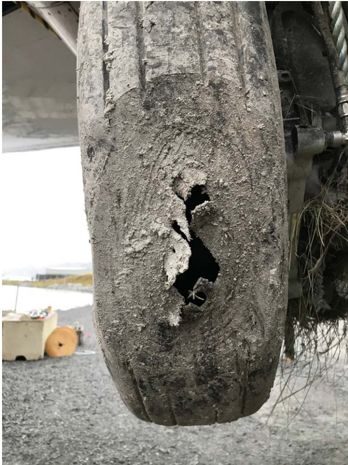
Figure 3 Damage to left outboard tire
