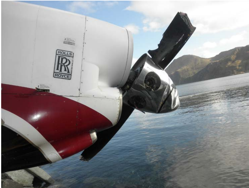
Figure 4 Damage to left propeller
