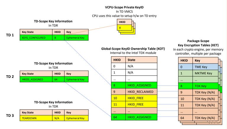
Figure 4.1: Overview of the Key Management State at TD-Scope, LP-Scope, Package-Scope and Global-Scope
