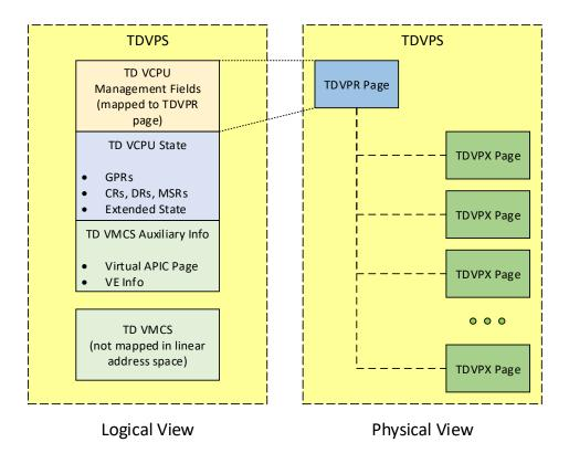
Figure 5.2: High Level Logical and Physical View of TDVPS
