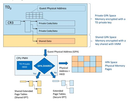
Figure 2.3: Secure EPT Concept
