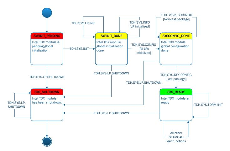
Figure 12.1: Intel TDX Module Lifecycle State Machine
