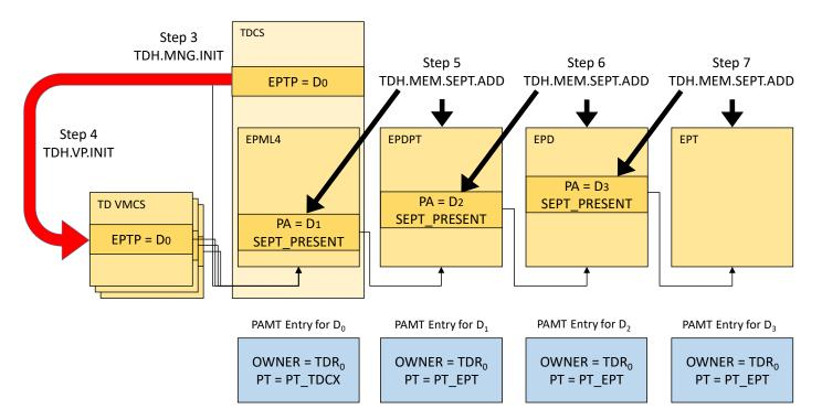
Figure 7.3: Typical Secure EPT Hierarchy Build Process
