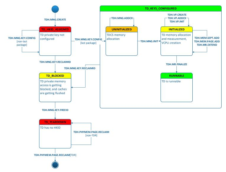
Figure 5.3: High-Level TD Life Cycle State Diagram
