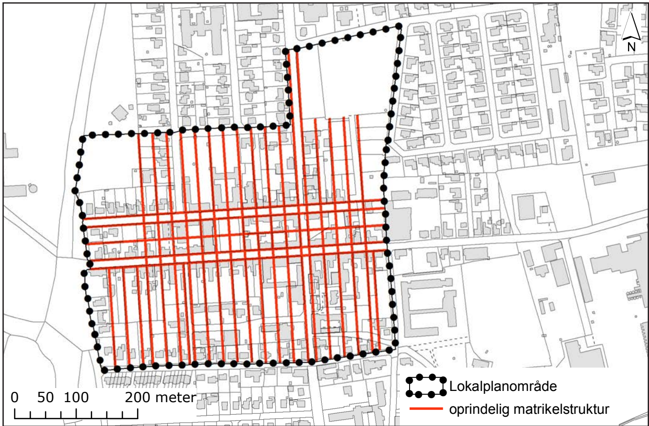
Map Annex 4 - Principle of the original plot structure. The structure follows old dimensions, a grid that measured 8x8 alen. A Hamburg alen is equivalent to 57.3 cm.
