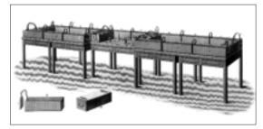
Battery which Davy used to discover elements such as sodium and potassium. Contemporary print
