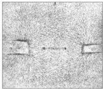
Iron filing diagram showing the structure of space near a magnet. Made by Faraday, early 1850s
