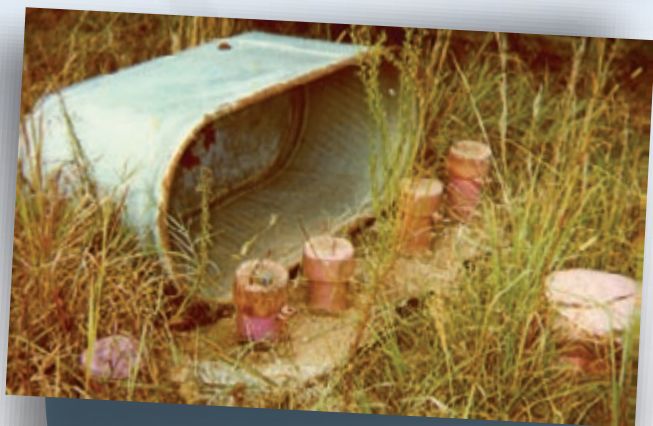
RECOVERED AMERICIUM FROM RETIRED WELL LOGGER, OKLAHOMA 1996
