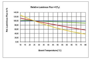
Figure 4: Relative luminous flux as function of board temperature for four different LED colors on ACULED®.
