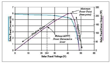
Figure 5: Relationship of the panel's current and power to its forward voltage.
