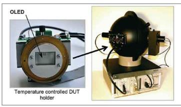
Figure 13: Integrating sphere with a temperature controlled DUT holder and the OLED device attached to it.
