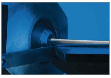
Figure 9: Extrusion is an economically viable process for mass production of rotationally symmetrical components such as rods and pipes. Lengths from 3mm up to 400mm are possible. The diameters for rods range from 0.5mm to 20mm, and in pipes diameters up to 40mm can be produced.
