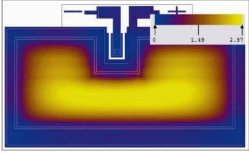
Figure 6: Temperature map of the active layer.
