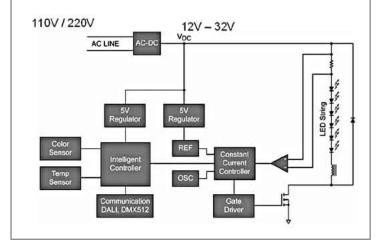
Figure 1: Standard, Single-Channel Lighting Design.
