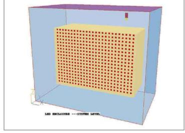
Figure 3: LED enclosure CFD Phoenics Model (red squares are the LEDs).
