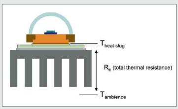
$R_{tt} = (T_heatslug - T_ambience) / heat emission LED.$
