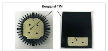
Figure 8: Bergquist GP2500S20 installed on heat sinks.
