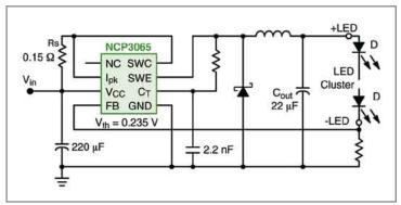
Figure 2: Typical schematic of a Buck Converter.
