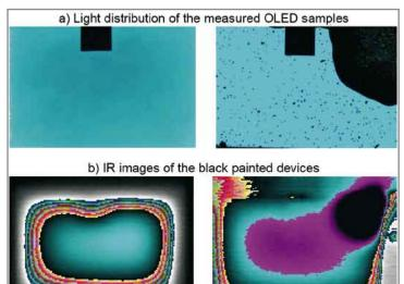
Figure 17: Light distribution and infrared image of a good and a faulty OLED sample to be used for validation of the thermal simulation model.
