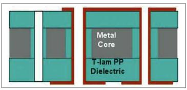
Figure 6: T-lam ML Metal Core Illustration
