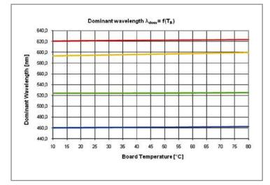
Figure 5: Dominant wavelength as a function of board temperature.
