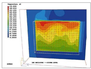
Figure 4: Temperatures in mid-enclosure plane for the case of no fans in still air using Phoenics.
