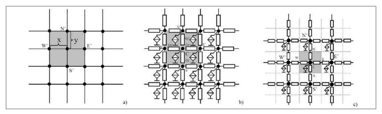
Figure 3: Models in 2D a) Finite differences grid b) Finite differences model c) Vector SUNRED model. - The description of the successive node reduction method can be found in earlier publications such as [3] and [10].
