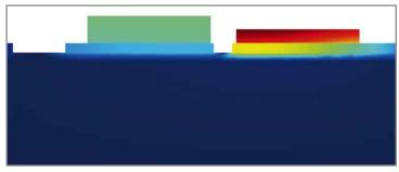
Figure 7: Thermal decoupling of the LEDs to avoid thermal crosstalk in the ACULED®.
