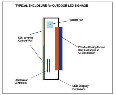
Figure 1: Typical enclosure for outdoor LED signage application.
