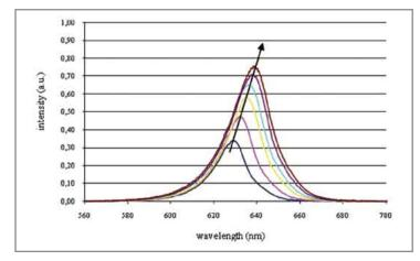
Figure 1: Wavelengthshift with rising LED junction temperature T<sub>i</sub>.
