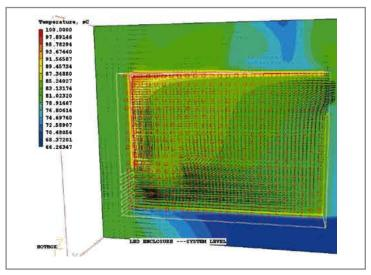
Figure 5: Temperatures in mid-enclosure plane for the case of 2 fans air using Phoenics.
