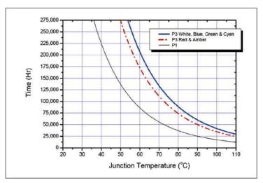
Figure 1: Lifetime vs. junction temperature (Source: Seoul Semiconductor Thermal Management Guide).
