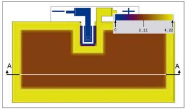
Figure 7: Potential distribution in the active layer
