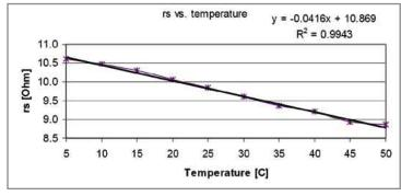
Figure 12: Temperature dependence of model parameter r.
