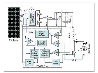
Figure 6: Schematic of a PV-LED streetlamp system using a single embedded controller.
