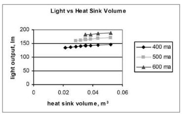
Figure 9: Light output versus heat sink material volume, junction temperature below 90°C.
