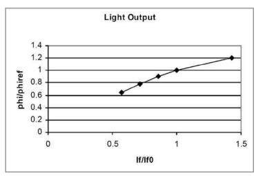
Figure 4: Relative light output as a function of current ratio.
