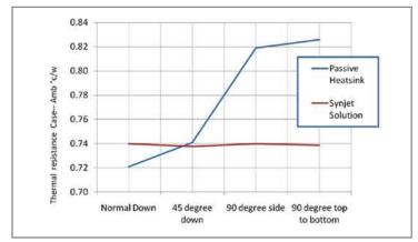
Figure 10: Thermal resistance in various heat sink orientations.
