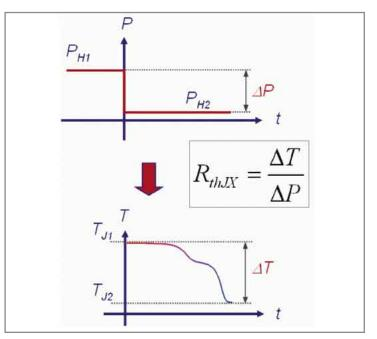
Figure 2: Junction-to-X thermal resistance calculated from a temporal difference of the junction temperature and the power dissipated in the device.
