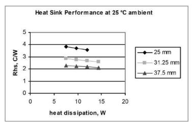
Figure 5: Heat sink thermal resistance as a function of dissipated power, various assembly depths.
