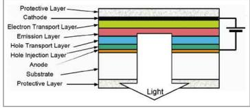
Figure 1: Typical structure of an OLED device [5]. The number of layers may vary.
