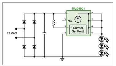
Figure 5: Typical schematic of a Constant Current Regulator.
