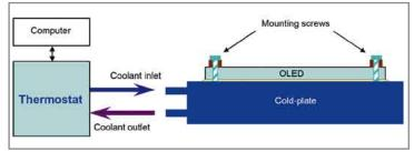
Figure 4: Measurement setup for measuring the I-V characteristics of OLEDs.
