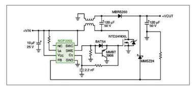
Figure 4: Typical schematic of a Buck-Boost (SEPIC) Converter.
