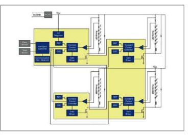
Figure 2: 4-channel lighting design with PowerPSoC. A single PowerPSoC device integrates all the devices within the shaded area.
