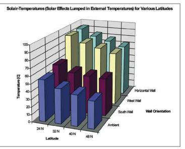
Figure 2: Typical Sol-Air temperatures for various latitudes.
