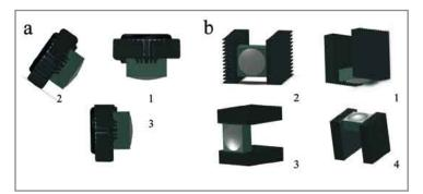
Figure 9: Active heat sink testing orientation (a - 1. normal down light position, 2. 45 degree, 3. 90 degree) and passive heat sink testing orientation (b - 1.normal down light position, 2. 90 degree side, 3. 90 degree top down, 4. down Light facing up).
