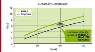
White LEDs in high heat dissipation PSML2 package
