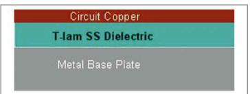
Figure 2: T-lam SS Construction
