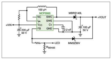
Figure 3: Typical schematic of a Boost Converter
