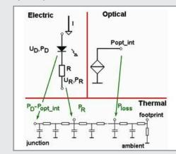
Figure8: Sketch of a multi-domain LED model
