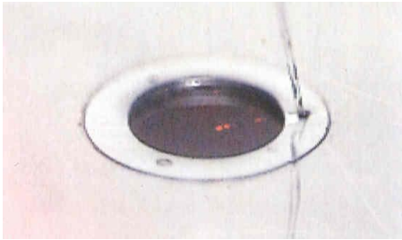
Fig. 13-7 Bottom element of Liquid-immersion objective.
