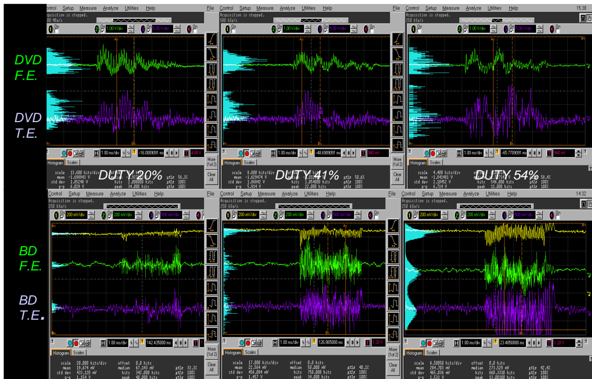
Fig. 6-5 Example of servo-error signals of DVD player and BD player
