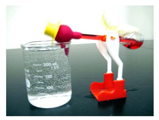
The Dippy Bird is made of **glass** filled with a fluid (methylene chloride), a gas phase (**Freon**, a chlorofluorocarbon) and a really penetrating **dye**. Take care of your Bird by keeping it in a place where it will be protected from strong sunlight and will not tip over. Furthermore, you should use distilled water in its dipping cup to avoid mineral stalactites developing on its lower bulb. Try not to get fingerprints on it, because that will interfere with its temperature exchanges.
