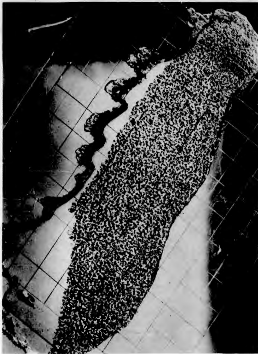
J5375 Fig. 10. Thick ice section examined under transmitted illumination (linear scale - centimeter grid).
