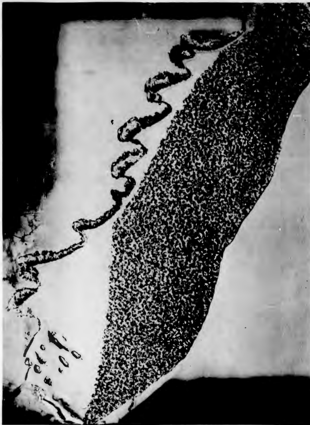
J5377 Fig. 12. Thin ice section examined under transmitted illumination (linear scale - centimeter grid).
