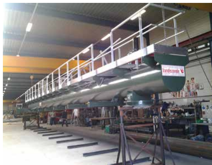
Scraper bridge - steel tube construction - tank diameter 15 m - Bastogne (Belgium)
