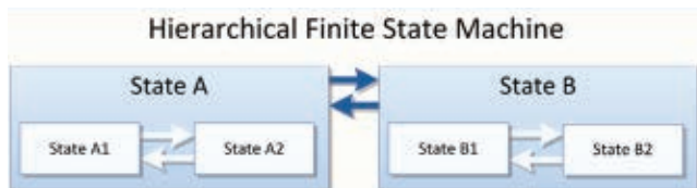
FIGURE 4: IN A HIERARCHICAL FINITE-STATE MACHINE, SOME STATES CONTAIN OTHER RELATED STATES MAKING THE ORGANIZATION MORE MANAGEABLE.
