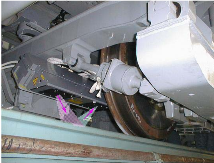
Figure 11: New optical rail displacement sensor
