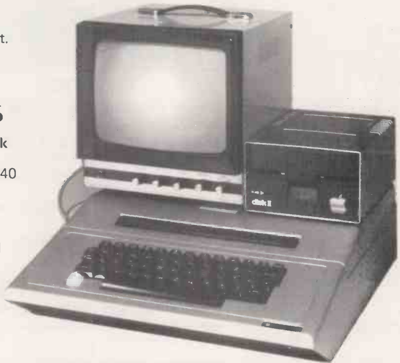
Photograph showing ITT 2020 with 9" Aztec Monitor and one 5¼" Disk Drive. (Price of £799 refers to 2020 only).
