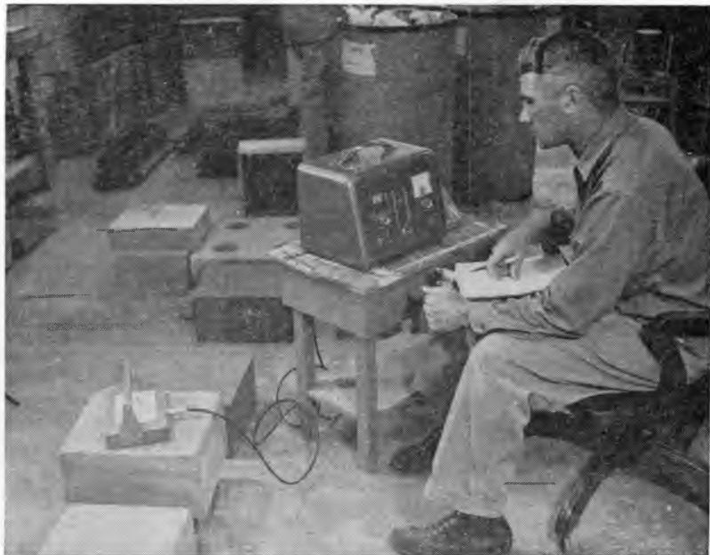
Fig. 7. A technician at the AASHO Road Test is shown running experimental tests on a gamma ray device which will be used to determine the density of materials. The test is nondestructive and much faster than conventional density tests.
