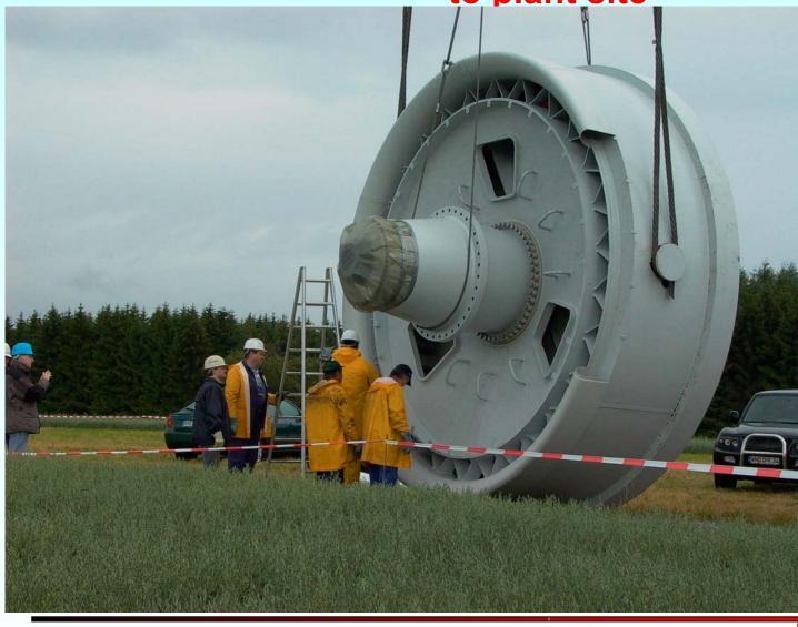
Outer PM rotor to increase torque by increased bore diameter
