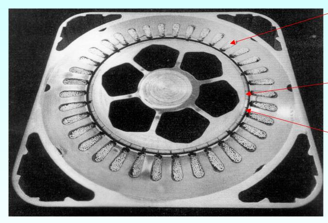
Stator slots with single layer winding, round wire
