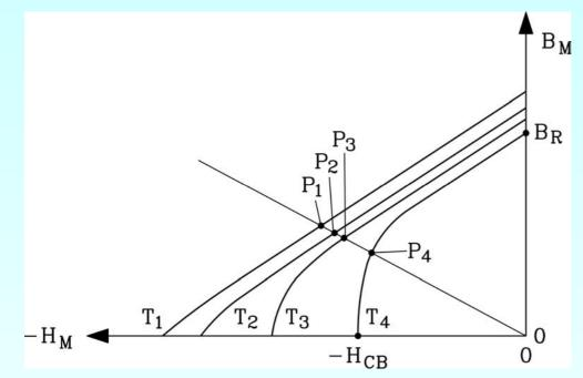
Determination of magnetic point of operation *P*:
