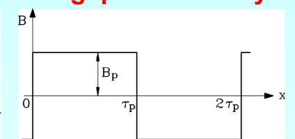
PM rotor with surface mounted magnets
