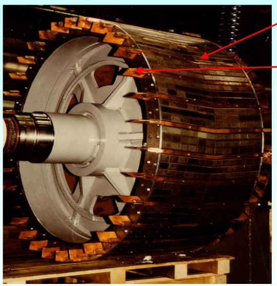
Skewed rotor magnets to reduce cogging torque
