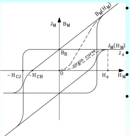
• Self-field of permanent magnets is called **magnetic polarization**  $J_{\rm M}$ , which adds to the external field  $H_{\rm M}$ , yielding the resulting flux density  $B_{\rm M}$ :
