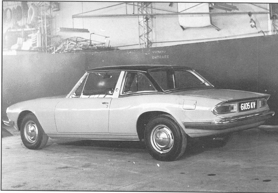
Michelotti's redesigned hard-top, shown fitted to the first Stag prototype, was a great improvement on the first design. A Standard-Triumph badge can be seen in the T-bar side member
