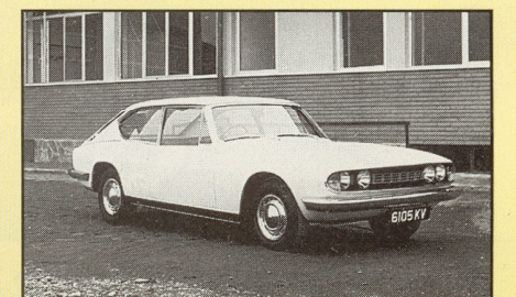
Below, the first fastback Stag, with an eggbox grille. The sliding headlamp covers had been abandoned by this time
