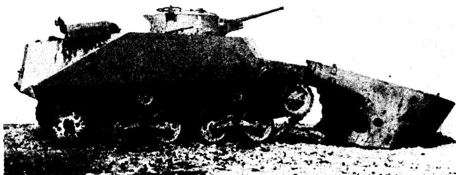
Figure 71.—Type 2 (1942) amphibious tank, releasing bow ponton.
