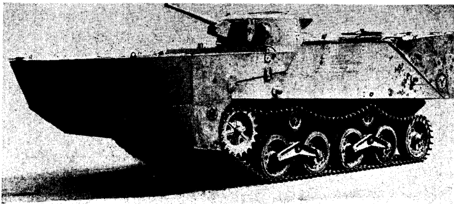
Figure 66.—Type 2 (1942) amphibious tank, left front three-quarters, with pontoons attached.
