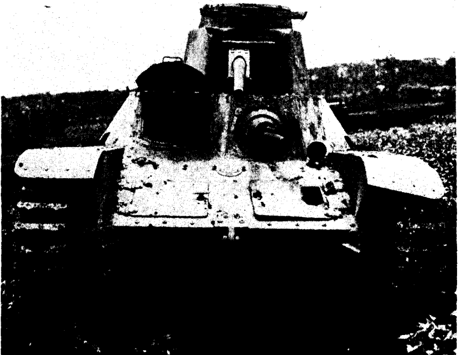
Figure 23.—View of a knocked-out Type 95 (1935) light tank showing the two hatches in the glacis plate and the driver's hatch.
