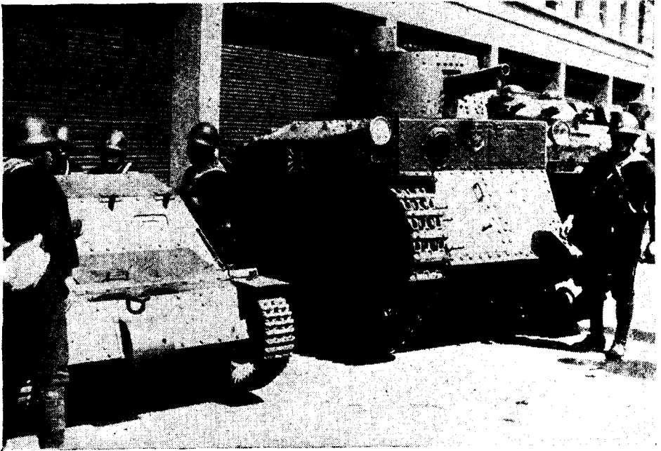
Figure 41.—Type 89A (1929) medium tank showing turret cupola. Note Navy insignia of anchor and chrysanthemum.
