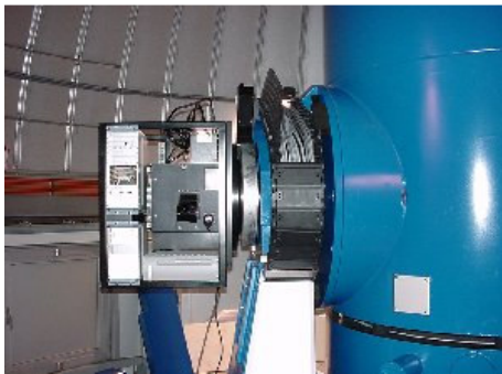
Figure 19: The Geneva photometer at the Mercator telescope
