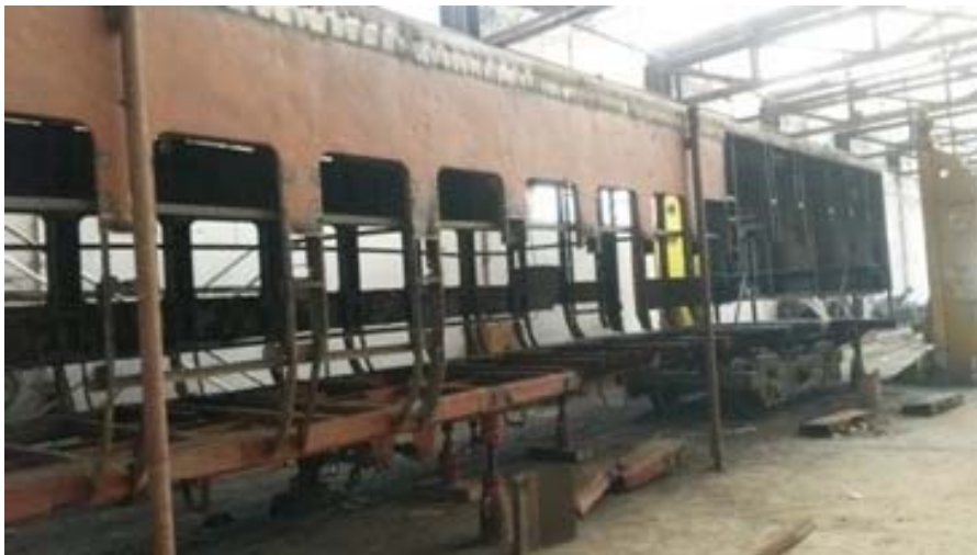
Figure 4-4: Coach Rebuilding under GOH at Railway Workshop, Saidpur
