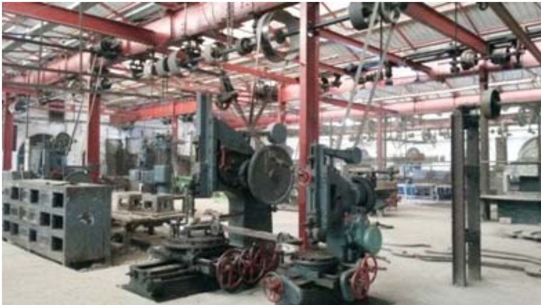
Figure 4-5: Belt Driven Machines in Railway Workshop, Saidpur
