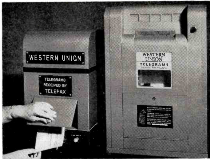
New Western Union Telefax unit (at left) alongside standard WU automatic telegraph machine.
