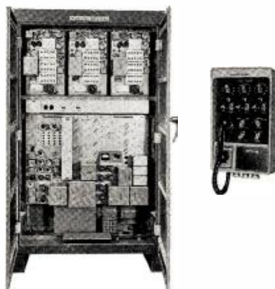
Left: Main cabinet of 248A equipment, mounting transmitter and three receivers. Right: Remote control unit.
