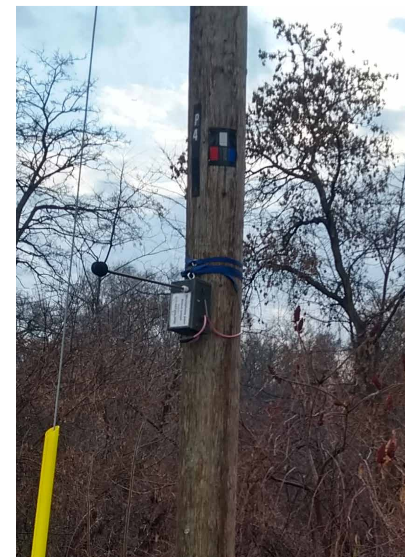
Noise logger capturing ambient noise
