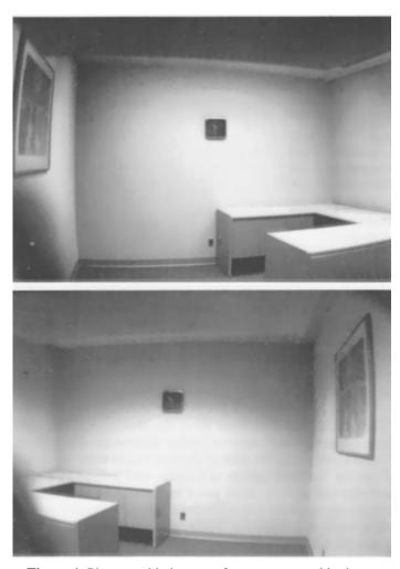
**Figure 1** Photographic images of two rooms used in the experiment: Top, a room having a relatively uniform distribution of luminance over the field of view; bottom, a room with a nonuniform distribution of luminance over the field of view
