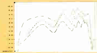
Fig 1. Klipsch Forte II: on-axis 1m response, with LF correction shown. Note separate additional traces for bass, mid and treble; dot/dash trace is near field correction
