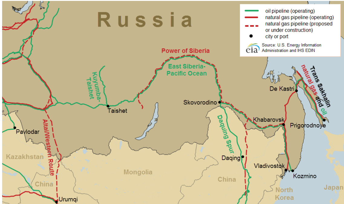
Figure 4. Major eastern Russian oil and natural gas pipelines
