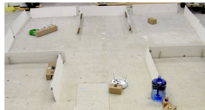
(d) The robots in depot 1 push the large box and the robot in depot 2 pushes a small box to the goal.
