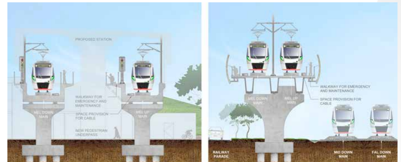
Figure 10: Typical track design cross sections at viaducts for Whiteman Park Station and Bayswater
