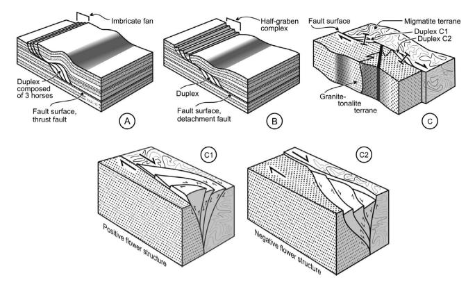
Figure 6. Duplexes form along deformation zones in various tectonic settings. They may be related to flat-lying (A and B) and steeply dipping (C) fault surfaces, respectively. Contractional and extensional duplexes are related to flat-lying fault surfaces. Positive (C1) and negative (C2) flower structures form along steeply dipping fault surfaces, strike-slip faults or strike-slip fault zones.
