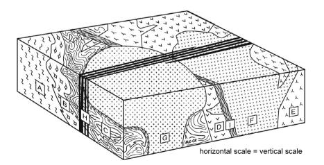
Figure 4. A hypothetical portion of crystalline crust such as that of Sweden. A – Gneissose granodiorite, B – augen gneiss, C – migmatitic lithic wackes (metatexites?), D – gabbro, E – diorite, F – tonalite, G – granite, H – dyke swarm, I – shear zone. Possible lithodemes: A, B, C, D, E, F, G, H and I. Possible igneous suite: D + E + F. Possible metamorphic suite: A + B + C. Possible dyke suite: H.
