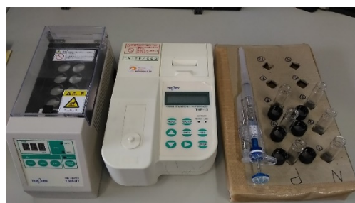
Fig. 2 Equipment for chemical analysis to measure Total Nitrogen (TN) concentration and Total Phosphorus (TP).
