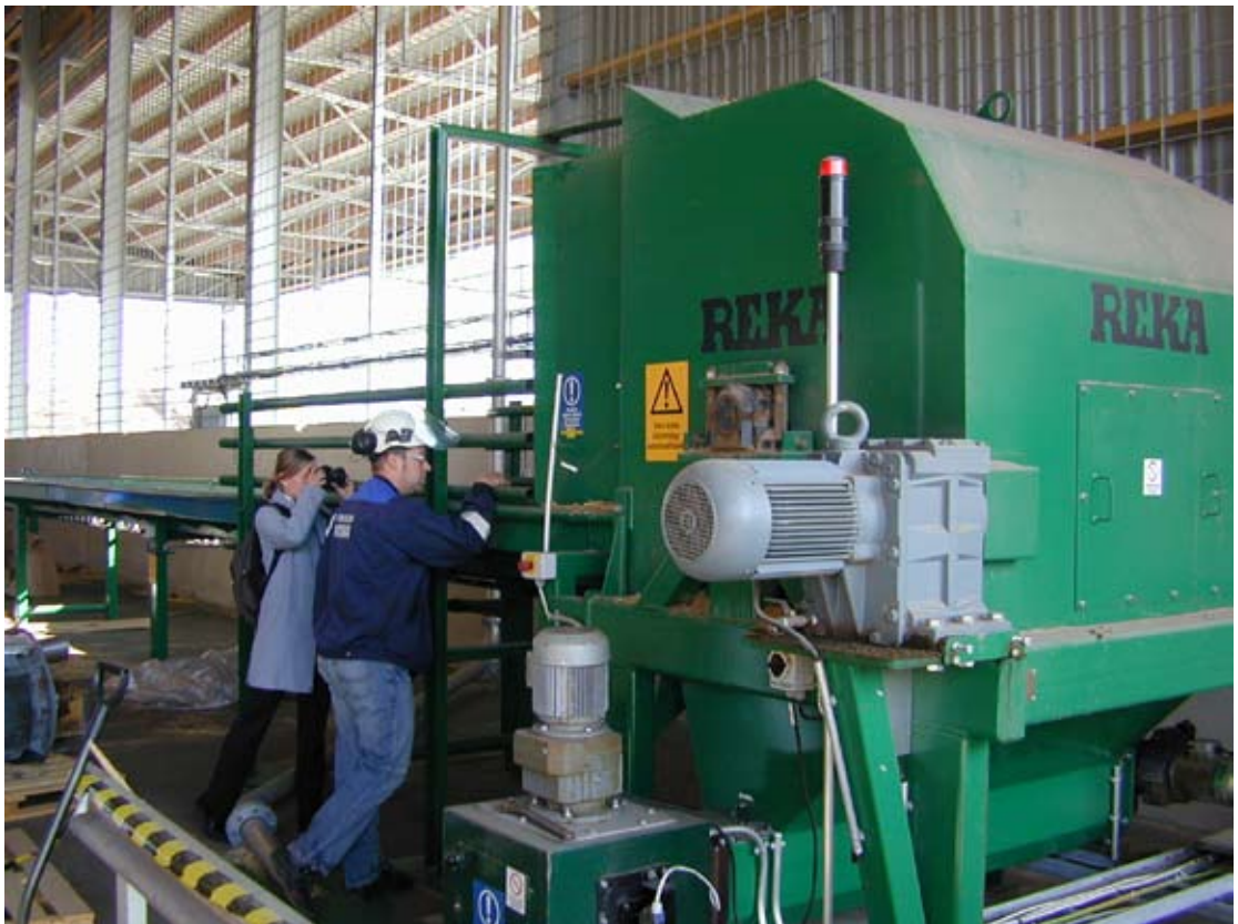
Utilisation of energy crops demands some investments in power plants, but these are not necessarily very costly. Above RCG-bale crusher line at Kokkolan Voima Ltd. (Photo: Timo Lötjönen, MTT).
