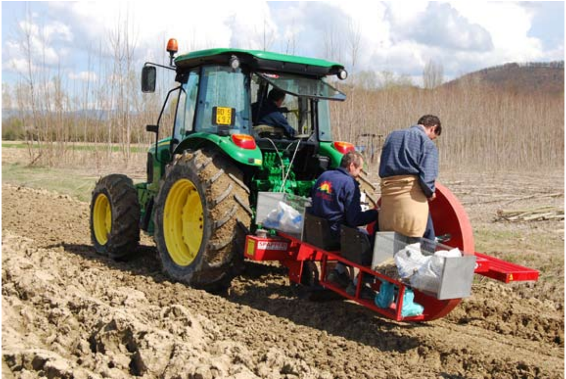
Poplar plantations are established with cuttings semi-automatically. (Photo: L. Corbella & M. Cocchi, ETA)
