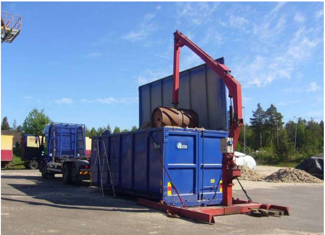
Compressing trials with spring-harvested hemp using a "Roll-pac" on. (Photo: Y. Söderström, Övik Energi AB).
