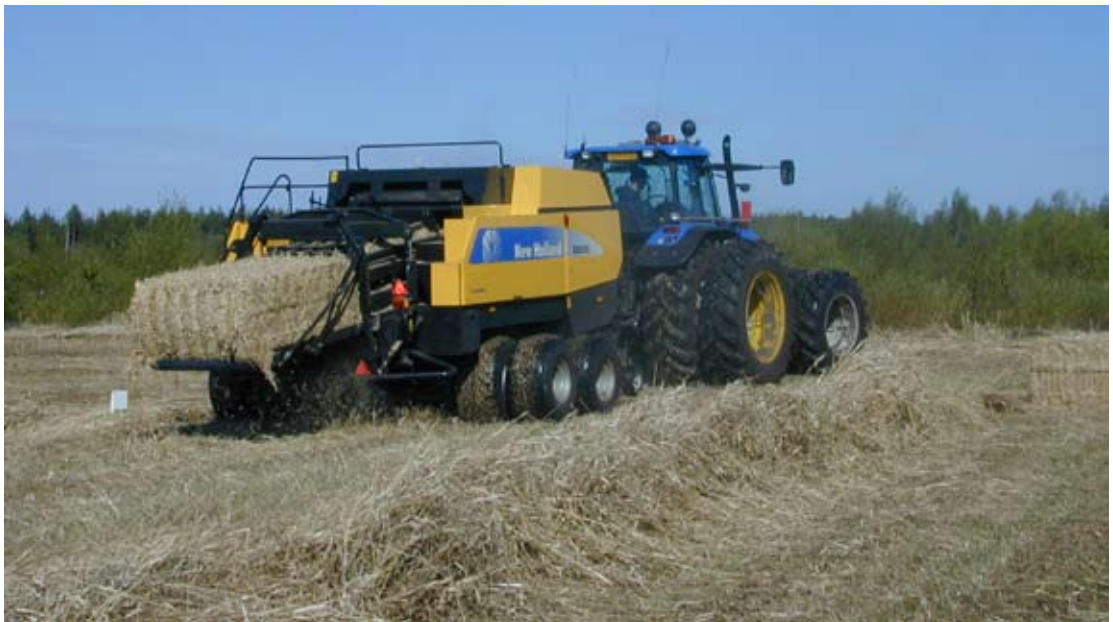
Advantages of a large square baler are the tight and well-shaped bales. (Photo: Timo Lötjönen, MTT)
