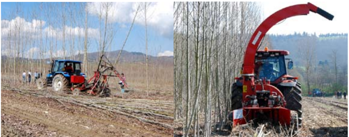
The Italian company Spapperi has developed harvest technology for small and medium scale poplar plantations. The trees are first cut down (on the left) and subsequently are chipped and blown into a transport trailer (on the right). (Photo: L. Corbella & M. Cocchi, ETA)
