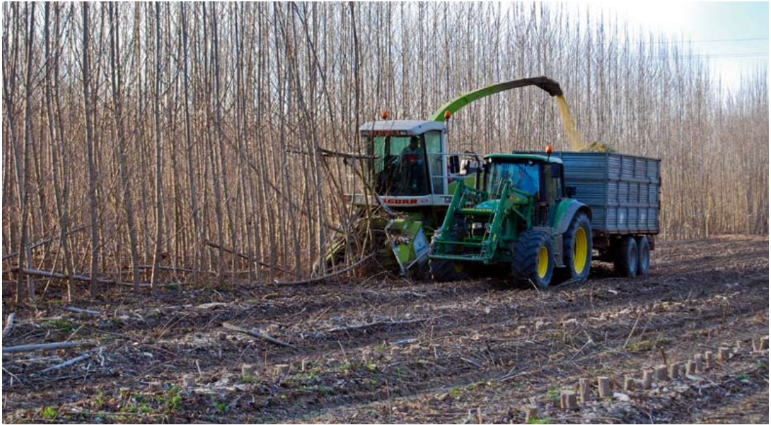
A modified self-propelled forage chopper cuts the poplars, makes woodchips and blows the chips into a transport trailer. (Photo: L. Corbella & M. Cocchi, ETA)
