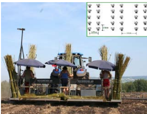
Twin row design for establishment of willow using a Step Planter. (Photo: Lantmännen Agroenergy AB)
