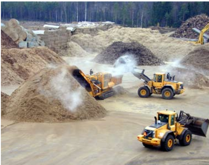
Preparation of reed canary grass-peat-wood mix with a wood crusher on the yard of a power plant. (Photo: Timo Lötjönen, MTT)
