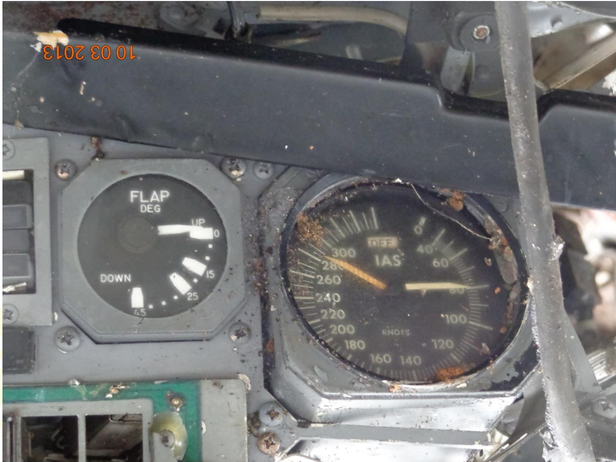
Figure 19: Flap Gauge Indicating 0°
