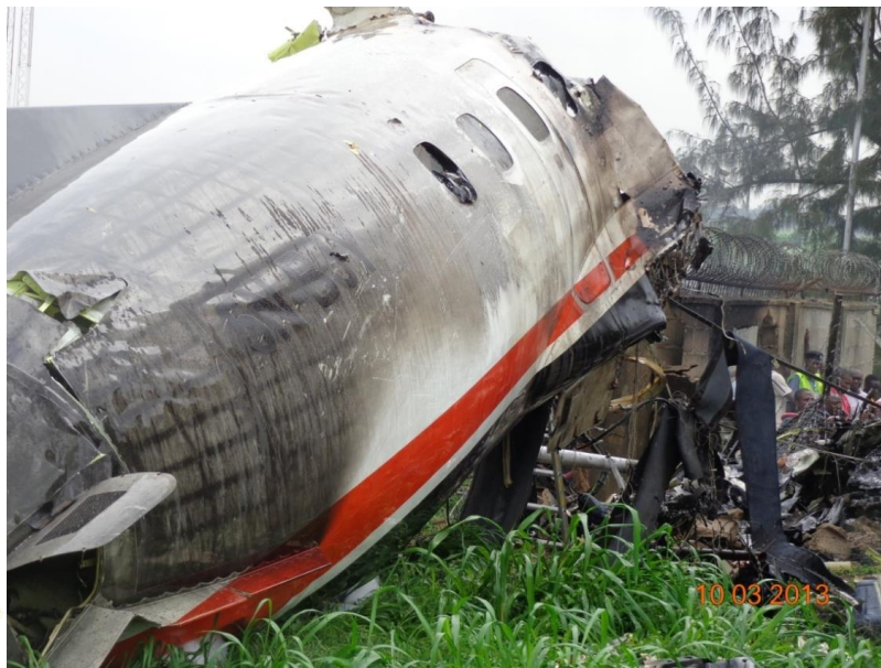
Figure 3: Aircraft rear section showing burnt areas
