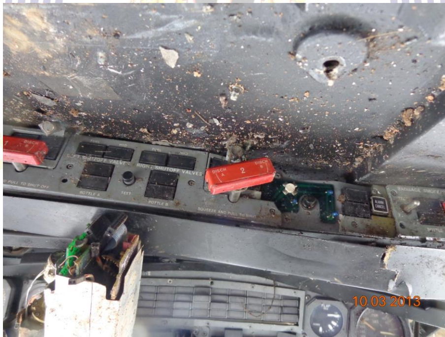
Figure 21: The No. 2 Fire Handle Pulled and Activated
