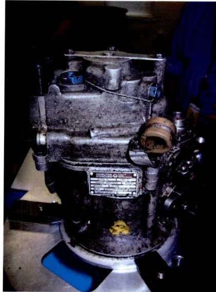
Figure 1. Propeller Control 871213 in as received condition.
