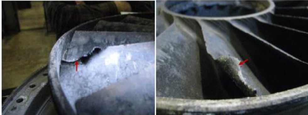
Photo no. 71 (Damaged vane L/E)
