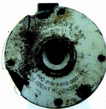
Figure 8 Electric Motor without Gasket or Coupler
