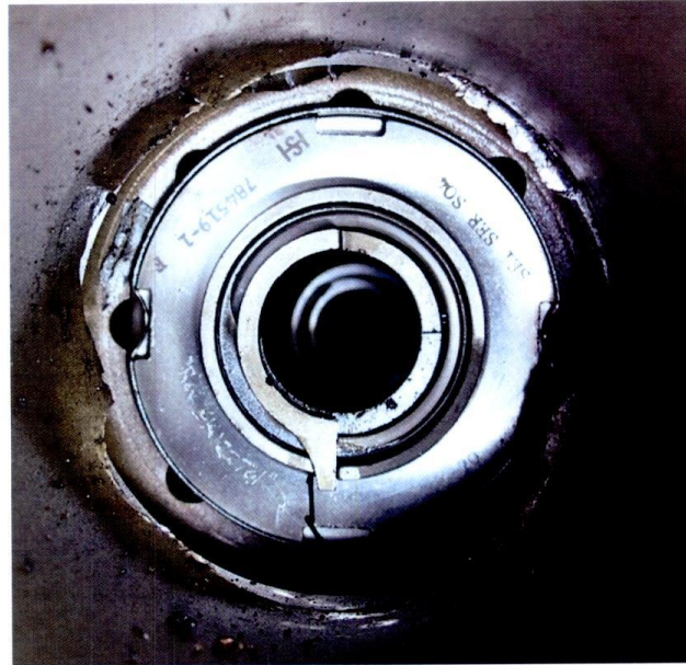
Figure 13. Broken Actuator Yoke Tailshaft.
