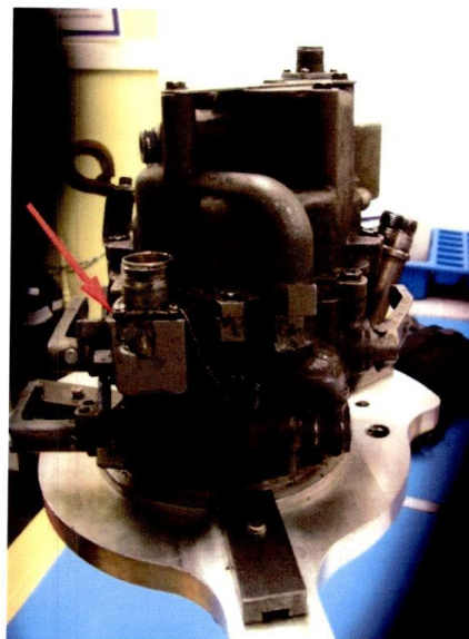
Figure 2. PCU Housing damage.
