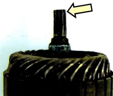
Figure 14 Motor Output Shaft Tip Bent
