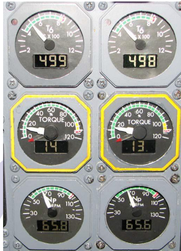
Figure 16: Engine Inter-turbine Temperature (T6) (top row) and Torque (centre row) Gauges and propeller RPM (NP) Gauges (bottom row).
