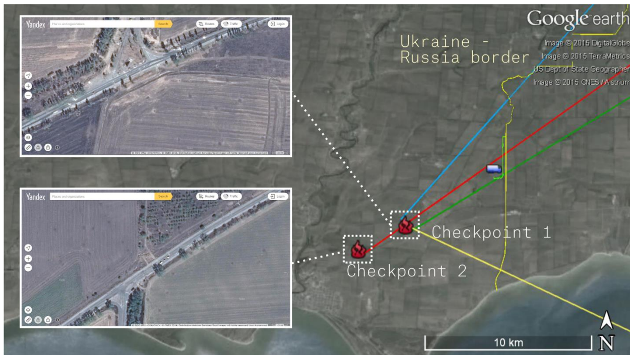
Figure 17. The position of artillery craters at Checkpoint 1 and 2 (47.149172, 38.159002 and 47.136150, 38.121798), and the average trajectories of fire as determined from crater analysis (straight blue, red, green and yellow lines, see Table 4 for further description of the craters). The trajectory of fire was determined from crater analysis, and the suspected firing point (47.180351, 38.228642) that shows three clear scorch marks facing in a southwesterly direction (see Figure 18 for further details). Satellite images of the artillery crater sites at Checkpoint 1 and 2 are stored in an online album 81 .
