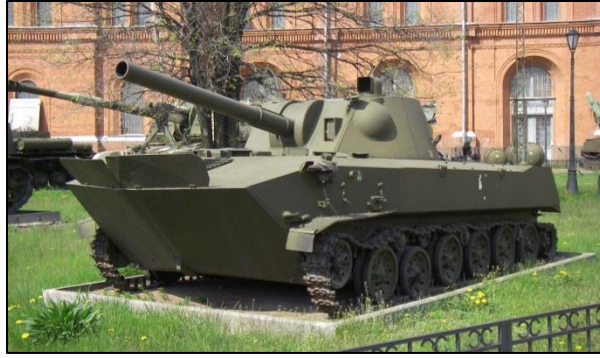
Figure 13. 120-mm self-propelled gun 2S9 'Nona' in Saint-Petersburg Artillery museum. Wikicommons 53 . This is the weapons system suspected of having been used in the artillery attack from Russia on 23 August 2014 (attack B).
