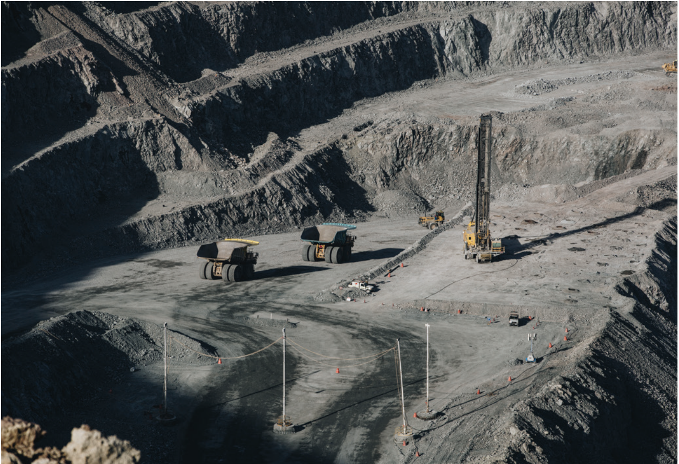
Drill and blasting area of the open pit mine, Oyu Tolgoi. The Oyu open pit is mined using conventional drill, blast load and haul methods.
