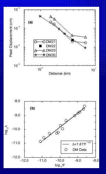
(1) Collect raw data from experiments: peak displacement versus distance.
