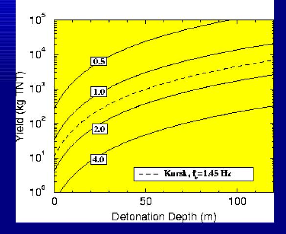
Quasi-analytic relationship between yield, depth, and bubble pulse frequency spacing. From WWII experiments.
