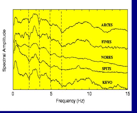
The spacing between peaks in the frequency domain is a function of yield and depth of detonation.
