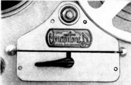
Top: The input and output jacks are found on a panel at the rear of the case. Lower, volume control in recording is gauged by the use of a "magic-eye" tube. Below this can be seen the tape motion control lever.
