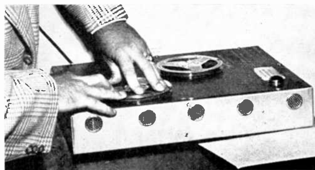
The tank-type Degausser is used in many places where there is a good quantity of erasing to be done, such as recording studios, radio stations, tape libraries, etc. The reels are placed on the panel, rotated and then very slowly withdrawn to complete the erase.
