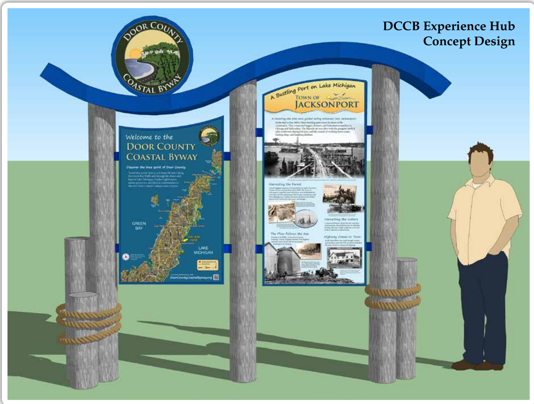
Hub has two panels 29.5" wide by 47.394" high and two panels 29.5" wide by 59.239" high, constructed out of 1/8"-thick high pressure laminate.
